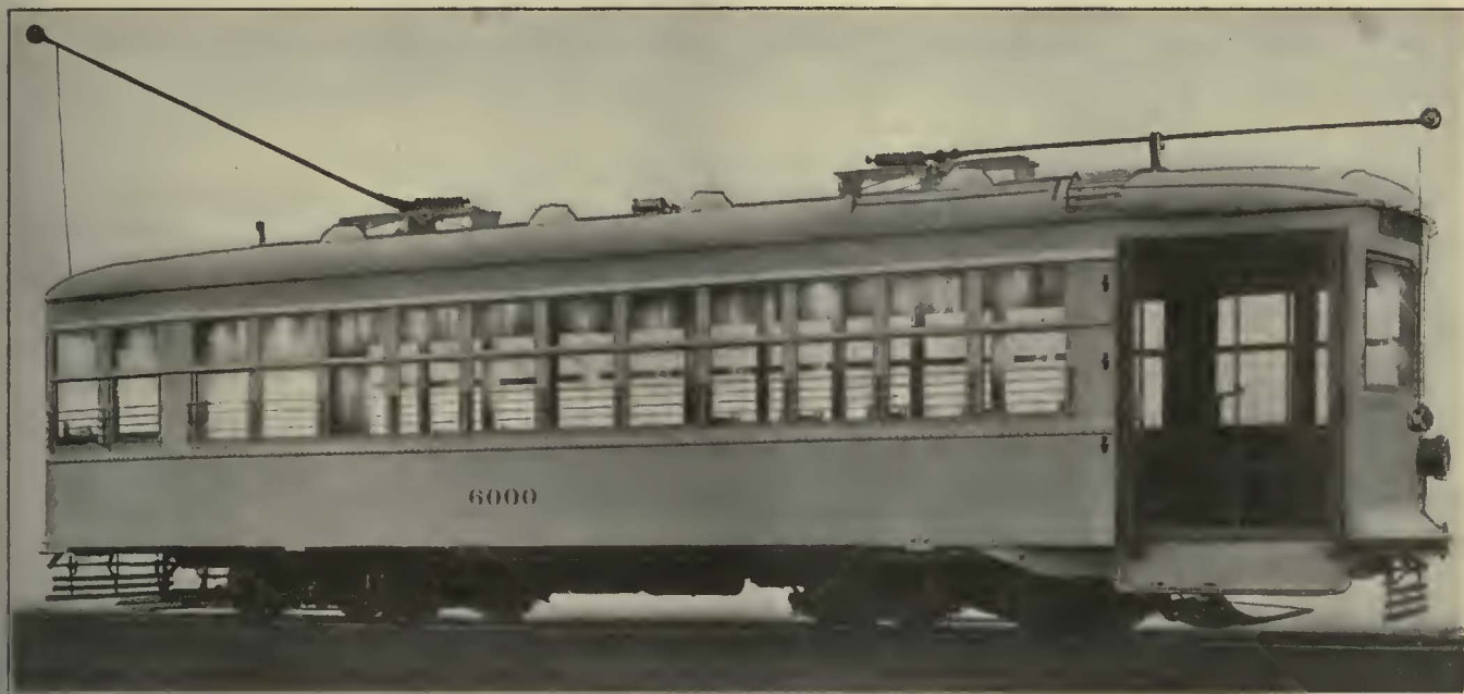
WIDE DOUBLE-DOOR OPENINGS FACILITATE ENTRANCE AND EXIT
