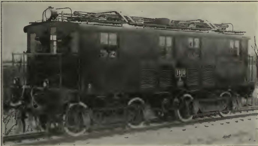
AT LEFT, 1,500-VOLT, 1,040-HP. LOCOMOTIVE FOR TRIAL USE OF JAPANESE GOVERNMENT RAILWAYS. AT RIGHT, INTERIOR OF OPERATING CAB, SHOWING LEFT-HAND DRIVE
