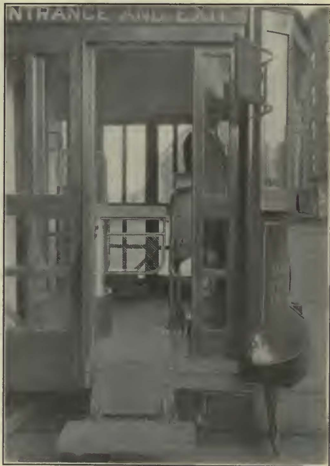
SLIDING DOORS AND FOLDING STEPS PROVIDE FOR ENTRANCE AND EXIT
