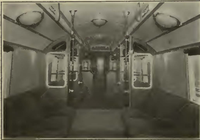
Car 821—Bowl Fittings Are Used for Lighting and Aluminum Trim Is Employed Quite Extensively
