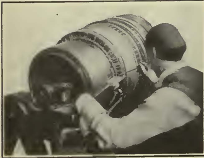
Soldering Leads at the Side of the Commutator
