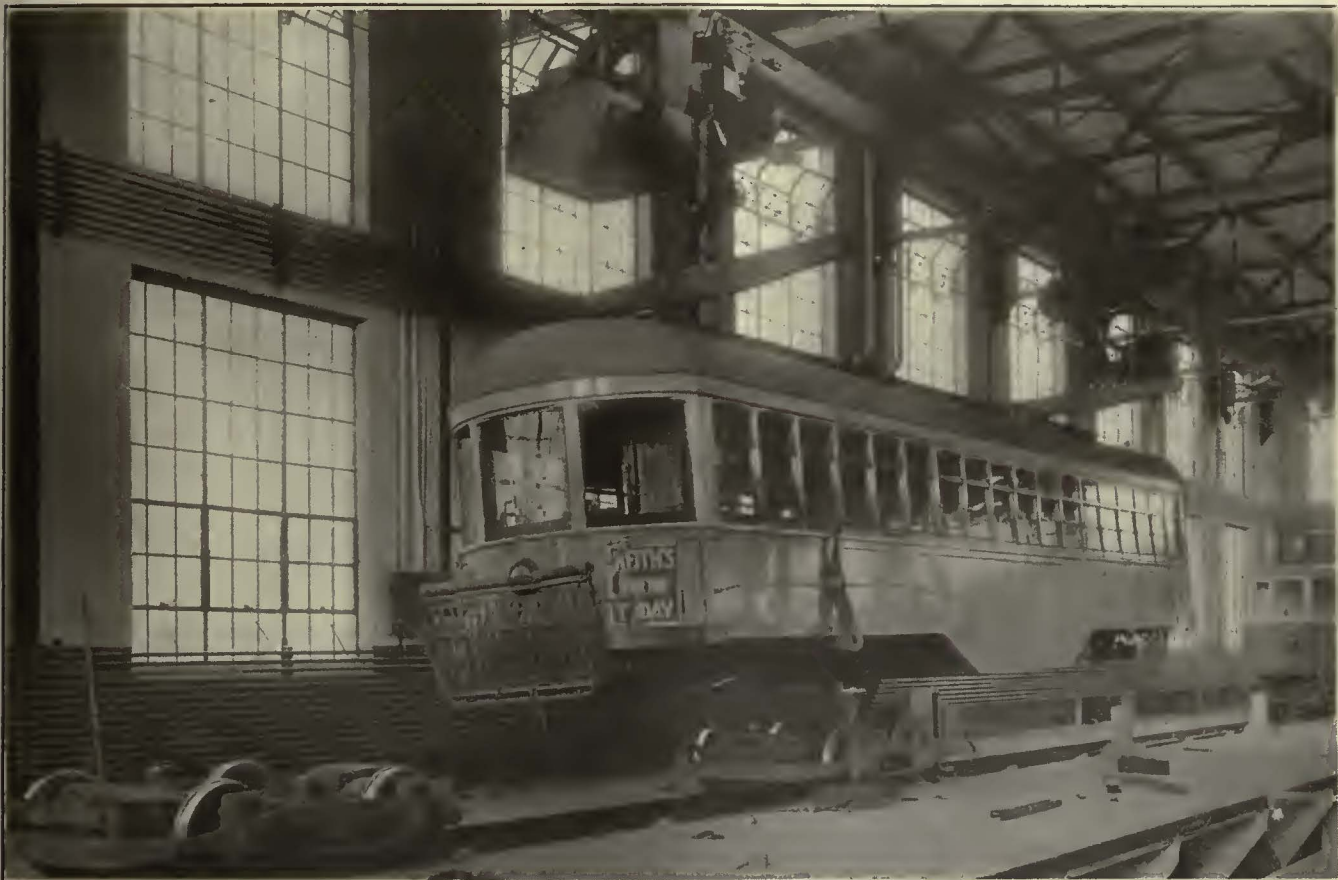
Lifting a Car Body by Means of Two Monorail Hoists in the Harvard Shops of the Cleveland Railway
