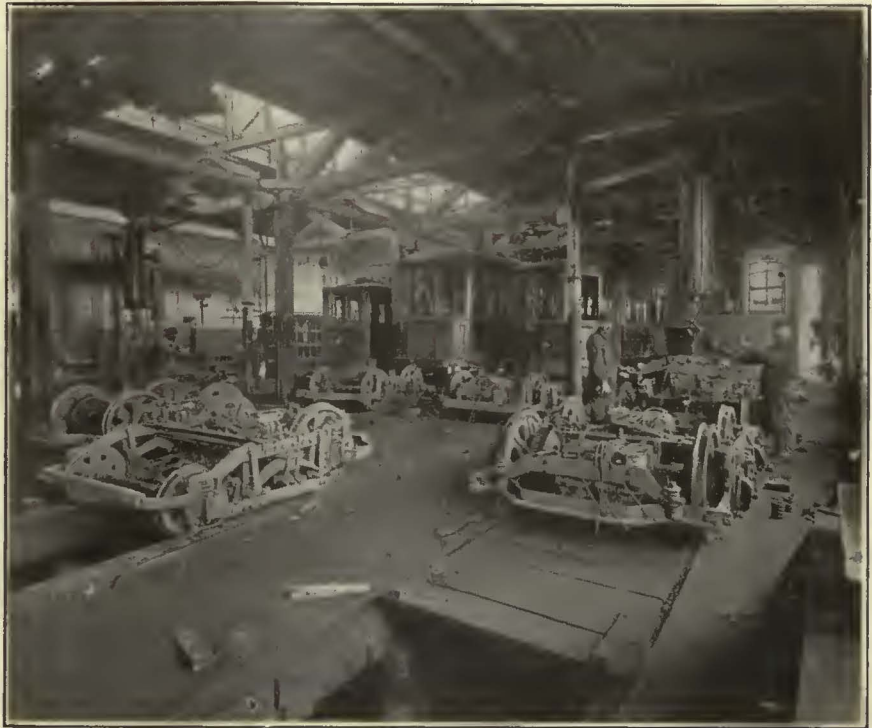
Overhauling Trucks in the St. Paul Shops of the New York State Railways, Rochester. Car Bodies Are Lifted by Chain Hoists, and Jib Cranes with Air Hoists Serve the Overhauling Floor
