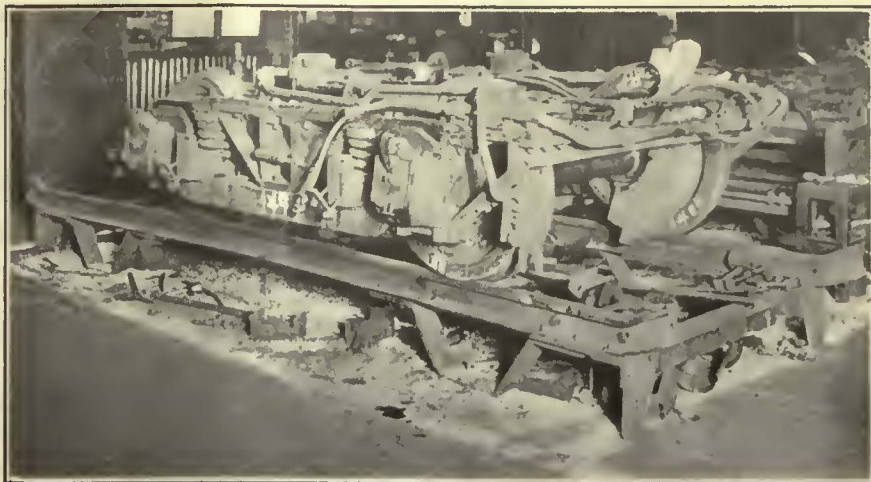
Truck Stand Enables Workmen to Accomplish Their Tasks with a Minimum of Physical Exertion and Time by Working in an Upright Position
