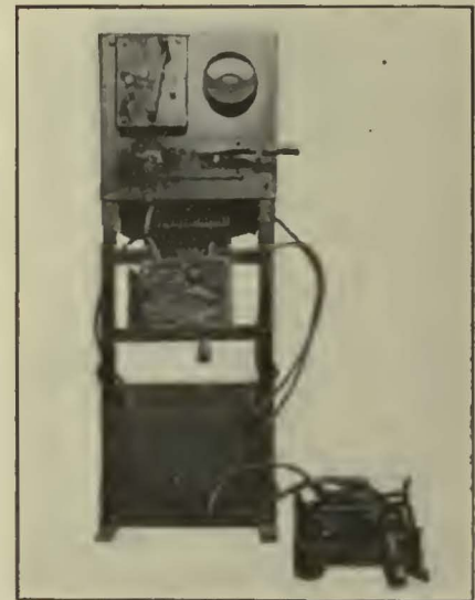
Circuit Breakers Are Tested with Storage Battery Current by This Board
