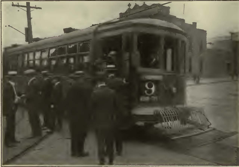
One of twelve large double truck cars of United Traction Company converted for one-man operation and in service on Pinehills and Country Club line, Albany, N. Y.
