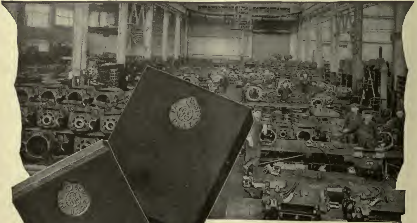
Section of assembly floor at Erie (Pa.) Works, where upwards of 5000 G-E Railway motors are built and tested annually.
