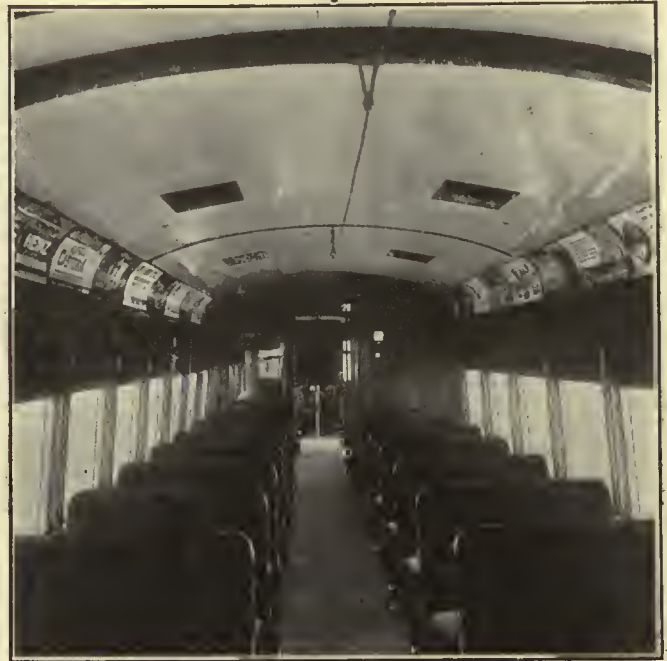
Two Compartments, Fabrikoid and Green Plush Seats, Center Toilet, No Bulkheads and Platform Floors Flush with Body Floor
