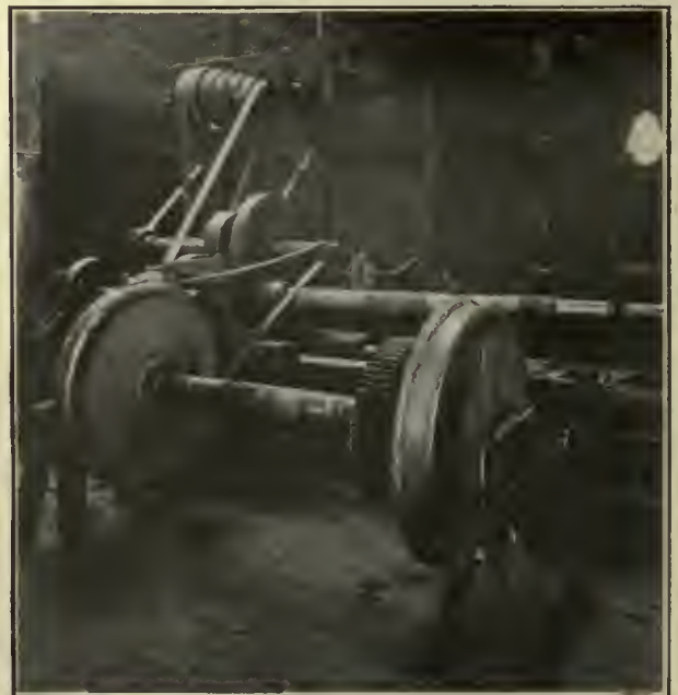
At Left, Belting Attachment to Old Lathe for Rotating Axle During Welding. At Right, Arrangement for Rotating Wheels for Building Up Flanges by Welding
