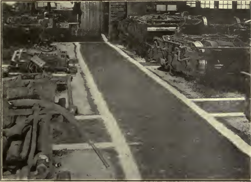
Truck Overhauling Shop Divided Into Sections by Whitewashed Lines
