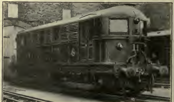
Photo by International News Reel Remodeled Electric Locomotive for Metropolitan Railway, England One-hour rating is 1,200 hp. at 600 volts and 30 m.p.h.
