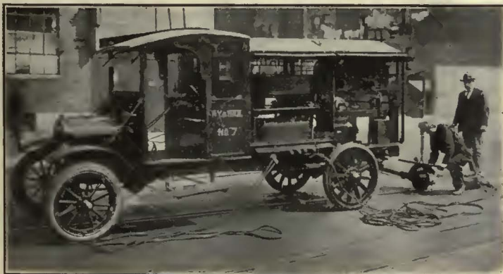
At Left—Receptacles for the Contact and Welding Leads Are Provided at the Lower Edge of the Chassis. At Right—Sheet Iron Curtains Close in the Equipment During Bad Weather and While Being Transported to and from the Job
