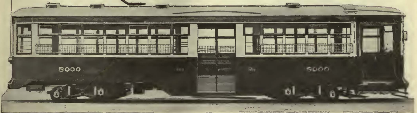
Sample Single-End Car of Which 385 Will Be Built for Philadelphia Rapid Transit Company
