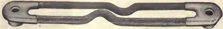
Pin Driven Terminal type of bond. For installing on web of rail under splice plate where space is limited. Made also in Compressed Terminal type. Cut shows special bond for very limited space. Type FP.
