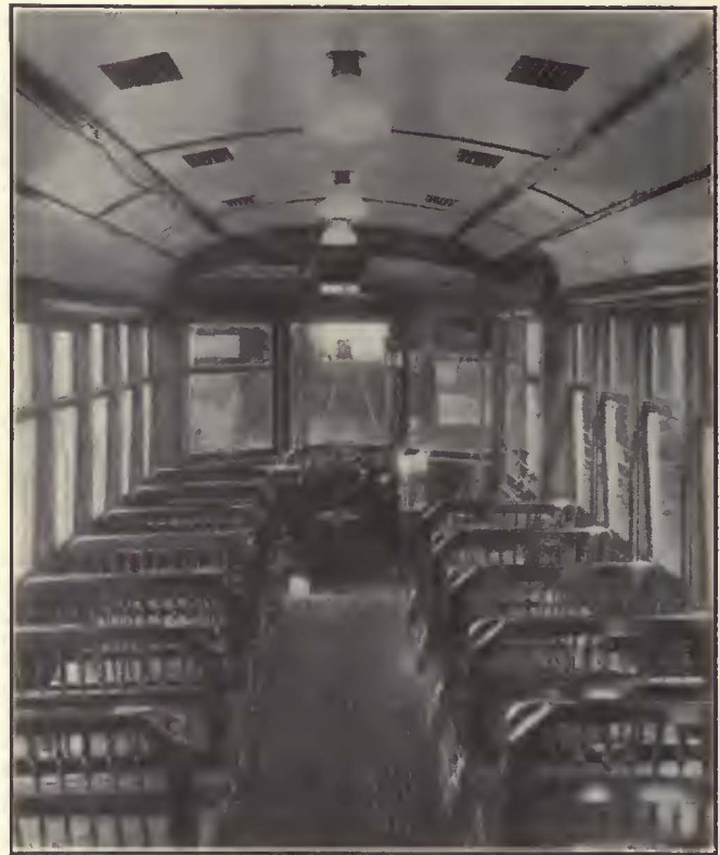
Interior of Older Type Car Rebuilt for One-Man Operation
