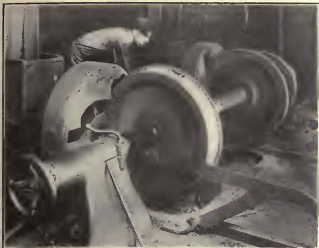
Grinding Out Flat Spots at the Sullivan Square Shop of the Boston Elevated Railway
