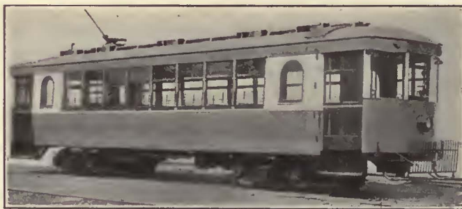
This Interurban Car for the Maumee Valley Railways & Light Company Weighs 25,000 Lb. and Seats Forty-nine Passengers
