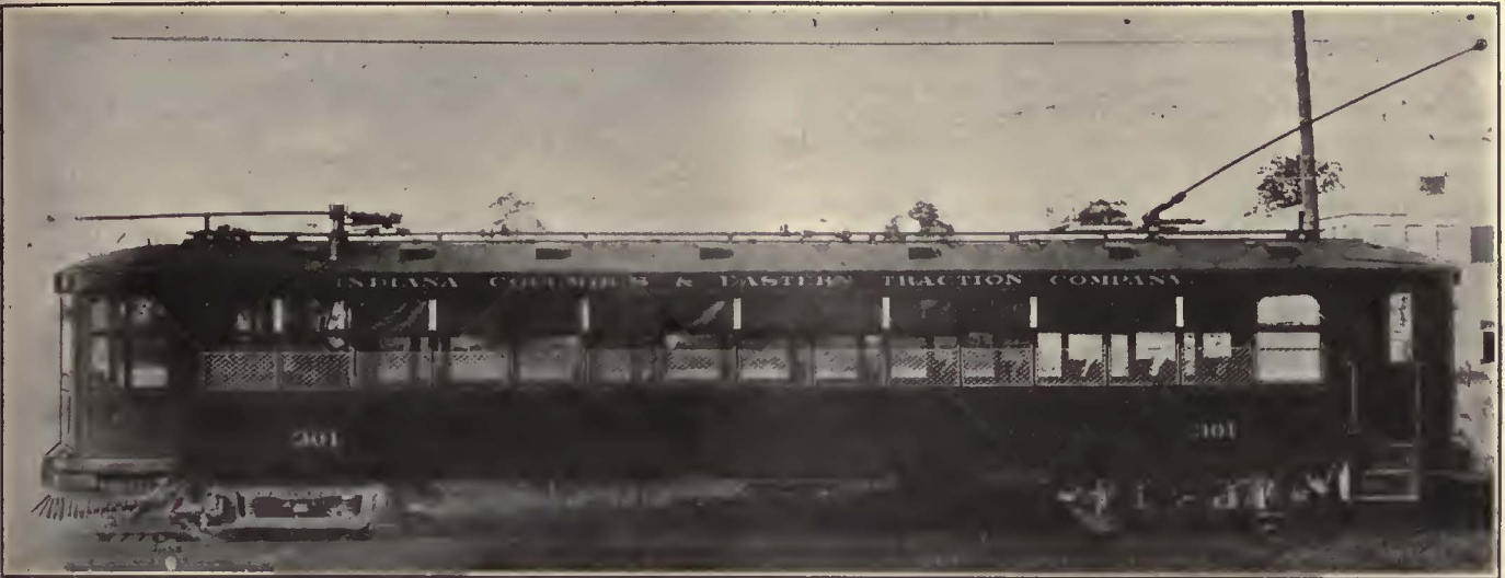
This 50,000-Lb. Interurban Car of the Indiana, Columbus & Eastern Traction Company Seats Fifty-eight and Has a Baggage Compartment. Its Free-Running Speed Is 55 M.P.H.
