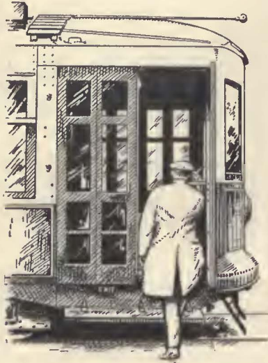
Showing Correct and Convenient Method of Passenger Interchange with Independent Door Control as Provided by the New SELECTOR VALVE.
