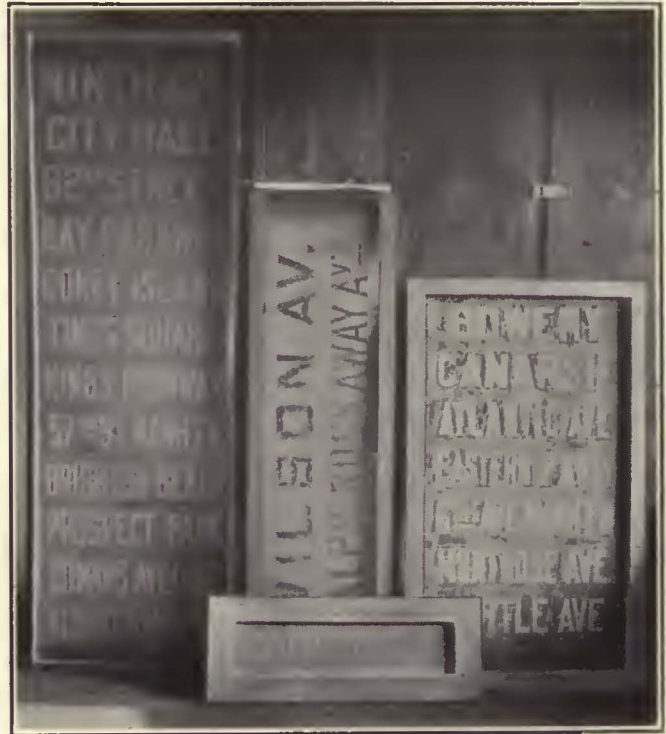
Several Sizes and Types of Silk Screen Stencils
