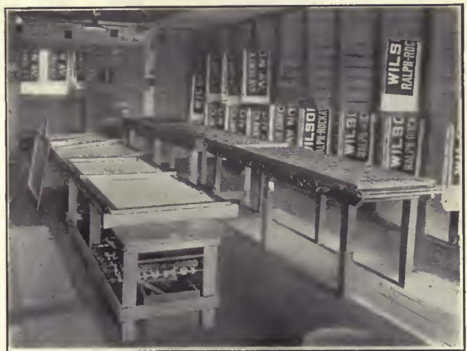
Lettering a Long Routing and Destination Sign by the Silk Screen Process
