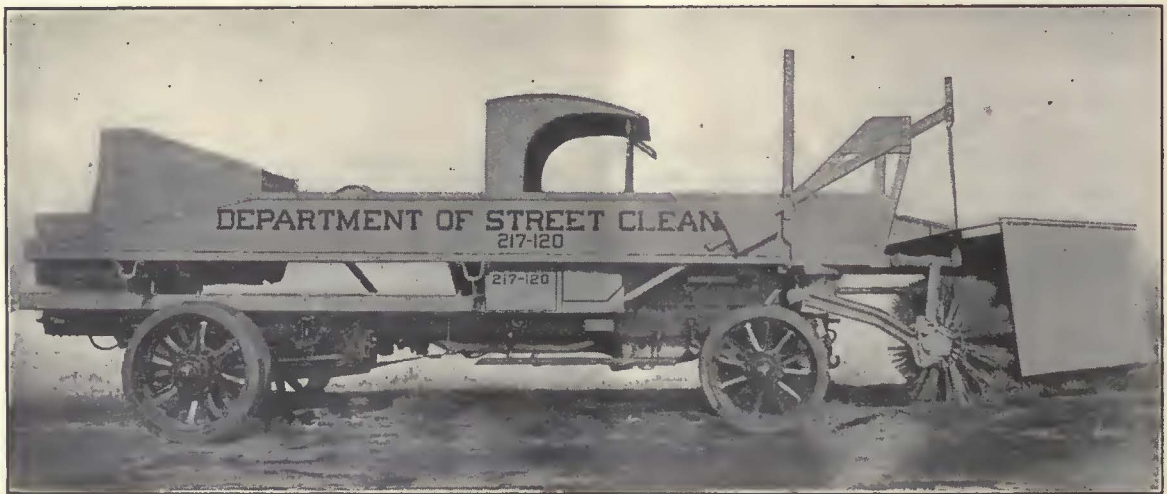
Rotary Snow Broom of type Used by Department of Plant and Structures on Staten Island Lines in New York
