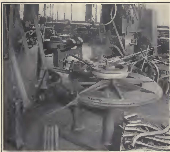
At Left, Belt-Driven Pipe Bending Machine. At Right, Power-Driven Machine for Bending Larger Sizes of Pipes and Structural Shapes
