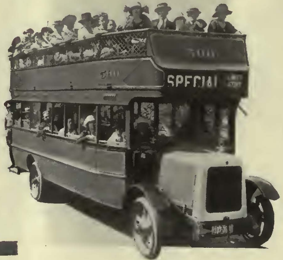
67-passenger double deck Yellow Coach now being built in large numbers for metropolitan service.
