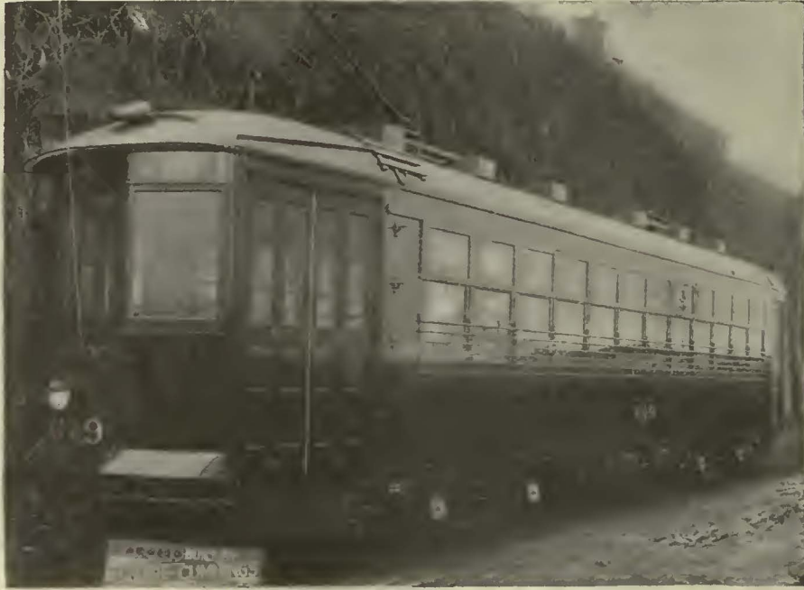
Multiple-unit-control double-track passenger car for two-man operation— Built for Georgia Ry. & Power Co., Atlanta.
