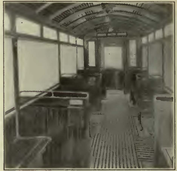
This Seating Arrangement Is Used Because the Car Is Only 7 Ft. 2 In. Wide
