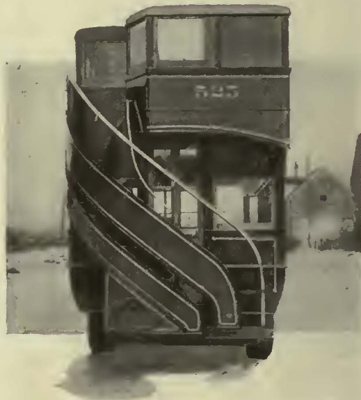
These three photographs show the Detroit type "Z," 67 passenger double deck coach with semi-enclosed top. This feature is of tremendous importance, the arrangement being such that top deck passengers have all the advantages of a full enclosure with none of the drawbacks.
