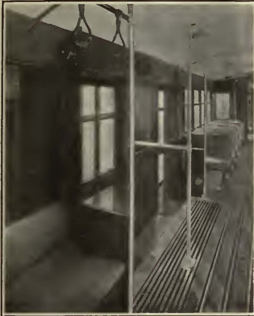
Stanchions Are Made of 1-In. Aluminum Pipe
