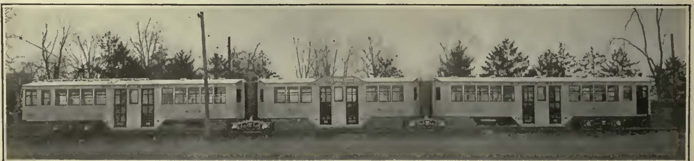
The Cylindrical Connecting Vestibules Between Cars Are Clearly Seen in This Broadside View
