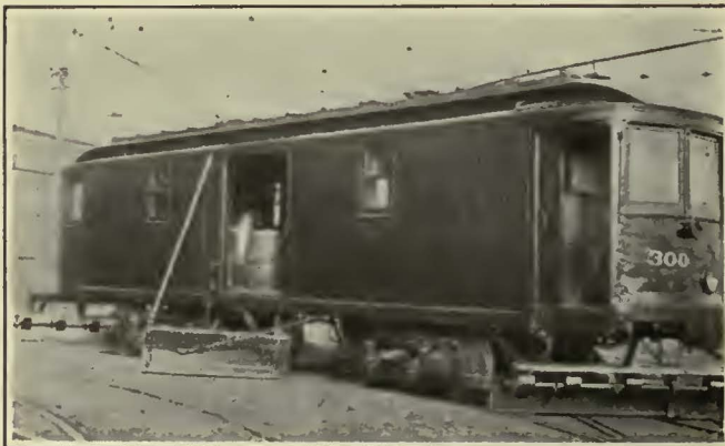
One of Several Express Cars Rebuilt by the Union Street Railway for Use as Snow Plows
