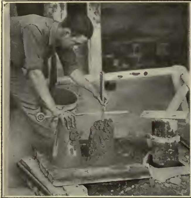
The Settlement of the Concrete Is an Accurate Indication of Its Consistency
