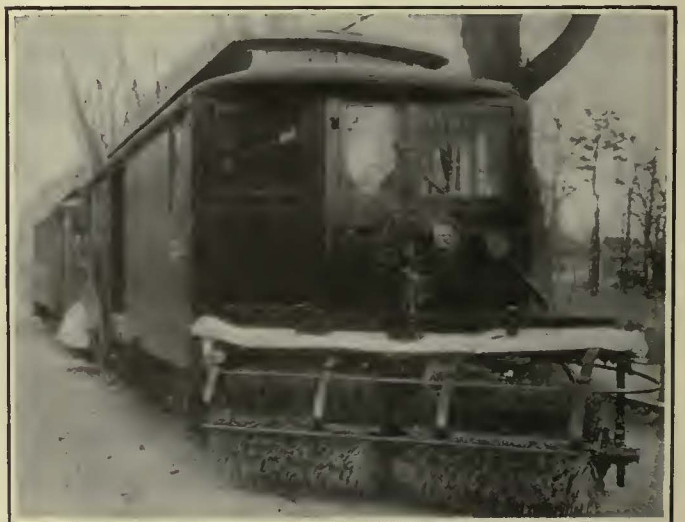
The Canvas Screen Is Fastened to a Metal Frame at the Top so that It Can Be Thrown Back When Desired
