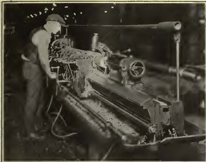
Machining a Large Subway Axle in a Lathe with Two Carriages and Six Tool Posts at One of the Shops of the Brooklyn-Manhattan Transit Corporation. The Illustration at the Right Shows Arrangement of Tools so that Six Surfaces on the Axle Are Finished at the Same Time
