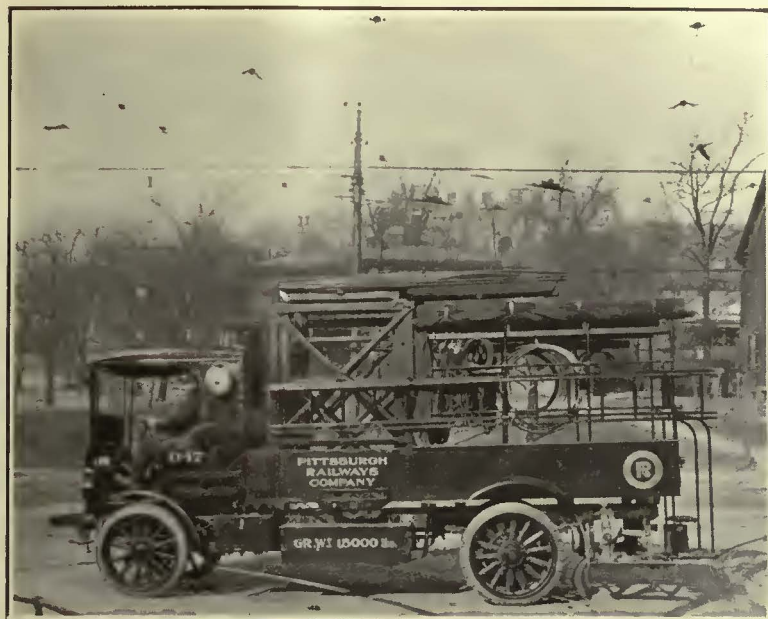
Latest Type Tower Truck Placed in Service by Pittsburgh Railways. Gross Weight of 15,000 Lb. is Marked on the Truck to Comply with the State Law. The Actual Gross Weight, Including Two Men, Was Found to Be 11,325 Lb.
