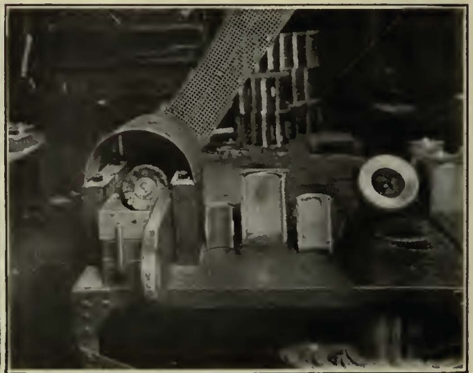
Left—Removing Excess Babbitt from Bearings with Circular Wire Brushes. Right—End View of Machine Shows the Brush and the Wedge Inserted to Remove Babbitt from Edge of Bearing
