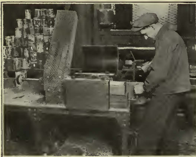
Left—Removing Excess Babbitt from Bearings with Circular Wire Brushes. Right—End View of Machine Shows the Brush and the Wedge Inserted to Remove Babbitt from Edge of Bearing
