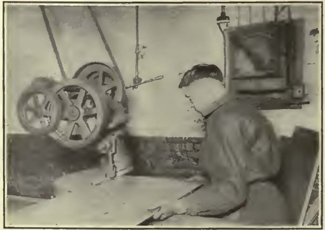
Serpentine Shear Handles Variety of Sheet Metals in C. S. L. Shop
