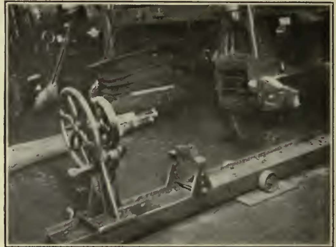
Left—Straightening an Axle on a 200-Ton Wheel Press at Harvard Shops, Cleveland. Right—The Fixture Used for Holding the Axle Between Centers While Being Straightened
