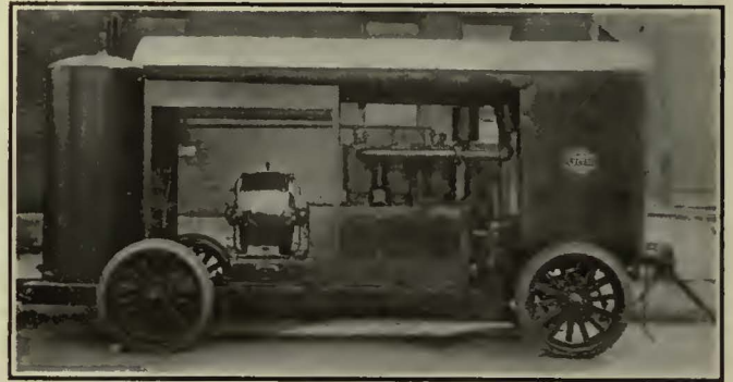
Rubber Tires and Spring Mounting Cut Maintenance Costs on Equipment
