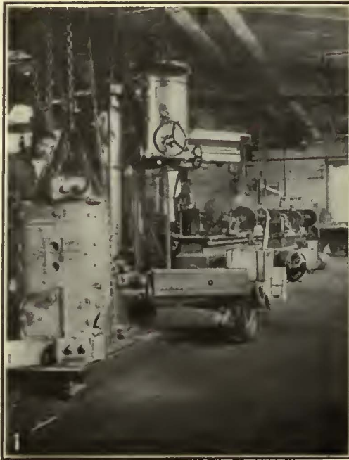
No. 1. Boring out a motor shell in the shops of the Washington Railway & Electric Company by use of a radial drill.
