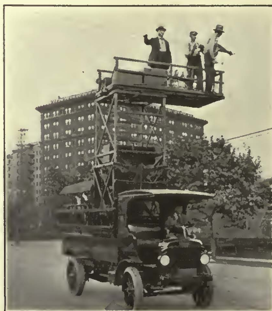
Latest Type Tower Truck Placed in Service by Pittsburgh Railways. Gross Weight of 15,000 Lb. is Marked on the Truck to Comply with the State Law. The Actual Gross Weight, Including Two Men, Was Found to Be 11,325 Lb.
