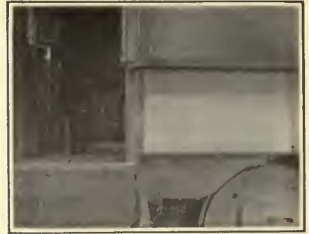
Galvanized Steel Panels Are Used to Protect the Woodwork on the Cars of the Middlesex & Boston Street Railway
