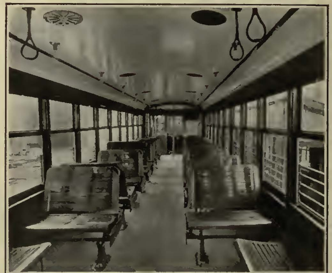
The Interior Has White Maple Floor, Mahogany Finished Seats and Trim and White Enamel Headlining
