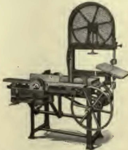
Woodworker with Positive Drive Ripsaw and Jointer Mandrel
