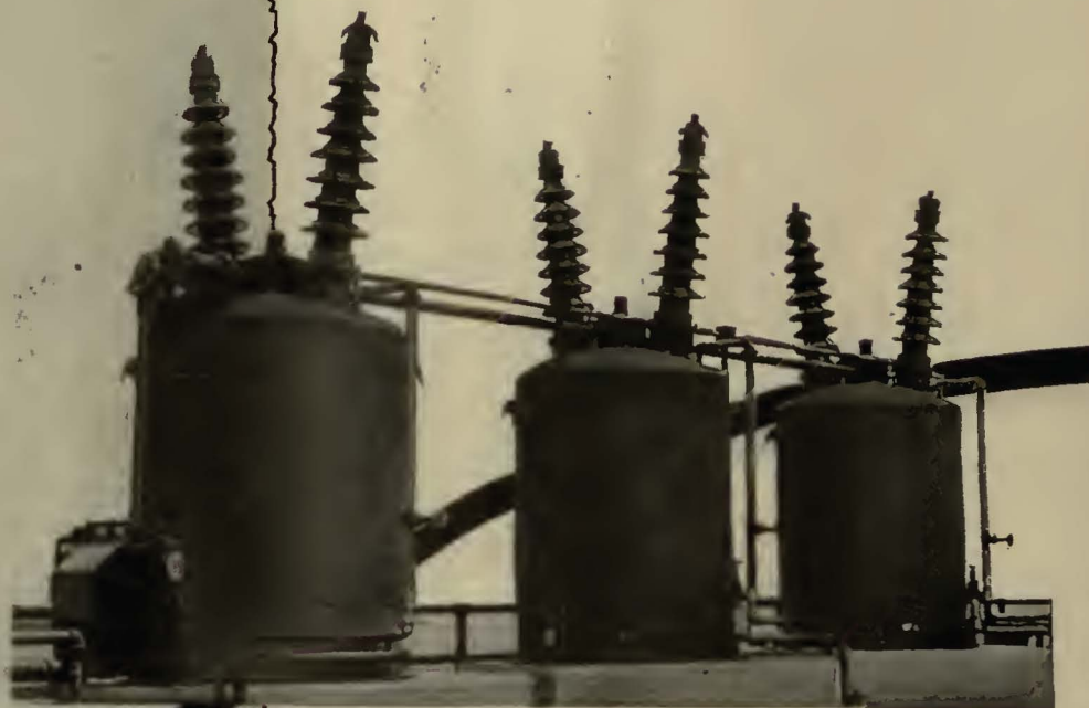
Type "G-2," 400 Ampere, 110,000 Volt, 3 Pole, Single Throw, Electrically Operated Floor Mounting Oil Circuit Breaker. Interrupting Capacity at Rated Voltage, 5300 Amperes.
