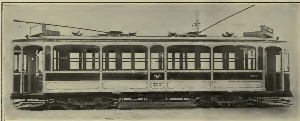
The Auckland Standard Car Has a Peculiar Arrangement of Sash, Inclosed Motorman's Compartment and Conspicuous Route Signs on Roof
