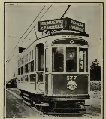
The Auckland Standard Car Has a Peculiar Arrangement of Sash, Inclosed Motorman's Compartment and Conspicuous Route Signs on Roof
