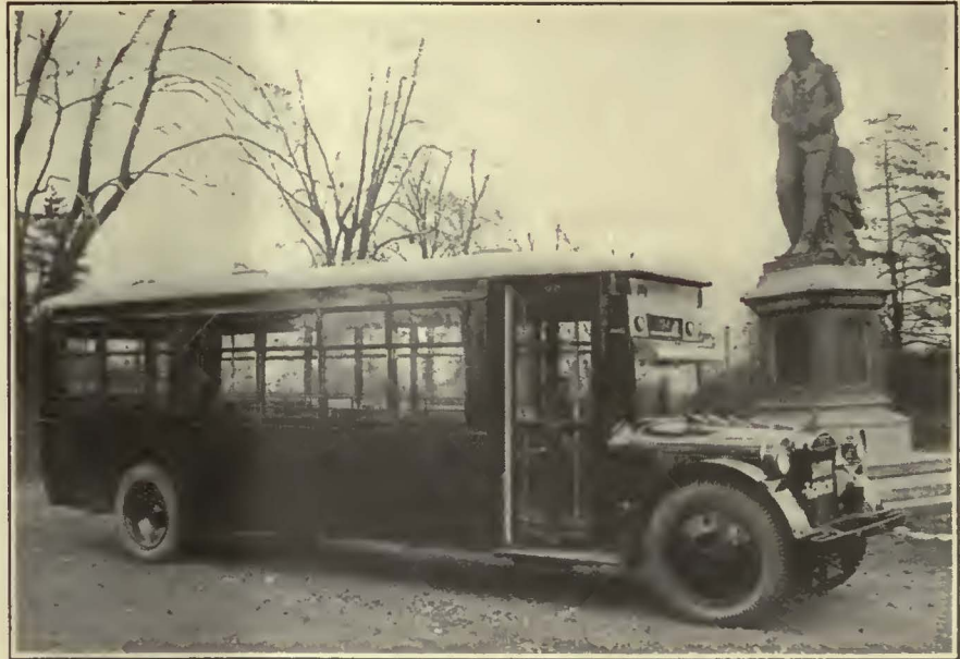
Birney Design Body Built by American Car Company on Fageol Chassis
