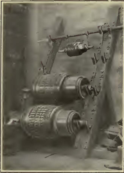
Built-In Armature Rack with Provisions for Supporting Short Armatures
