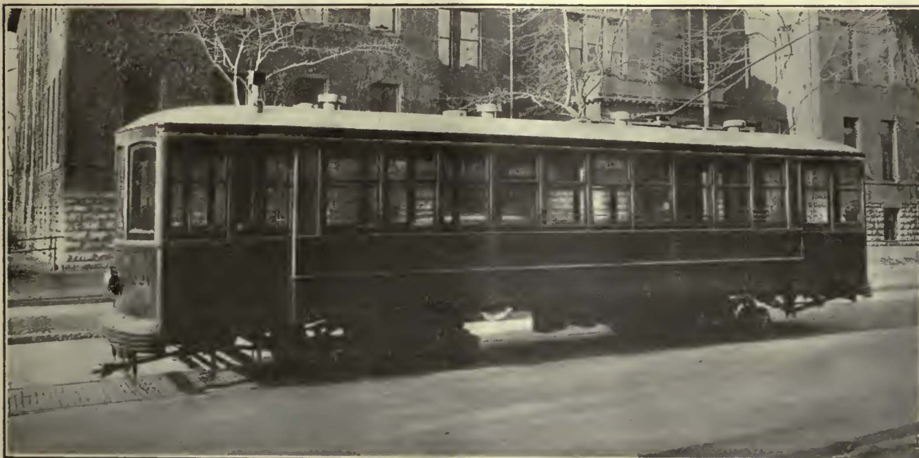
Double-Truck, Two-Man Car Rebuilt for One-Man Operation and Equipped with Safety Car Devices
