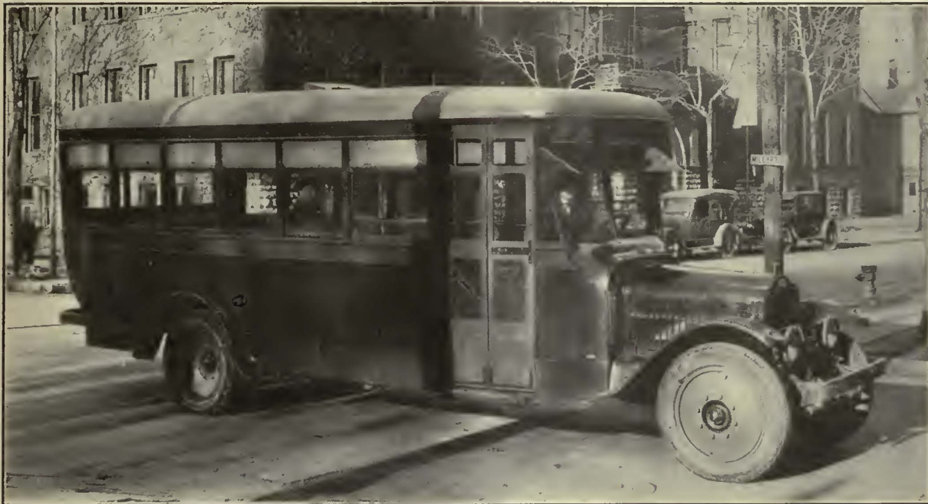
Twenty-five-Passenger, Street Car Type White Bus, Used on Car-Bus System of Saginaw
