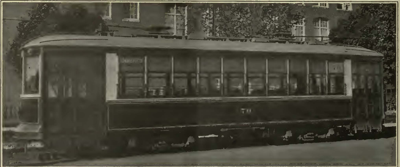
Double Track Safety Car for one-man or two-man operation. Built for Danville Traction & Power Co., Danville, Va.
