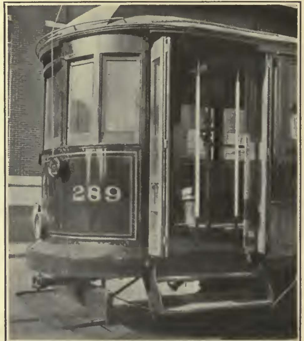
An 18-In. Section Was Added to the Platform to Fit New Bedford Car for Use on the Prepayment Plan. At Right, Enameled Stanchions Placed to Aid Ingress and Egress and Divide Passenger Streams
