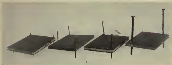
Note the resistance to splitting when nails are driven close to the edge. HASKELITE is easy to work with and contributes to the stability of the construction.
