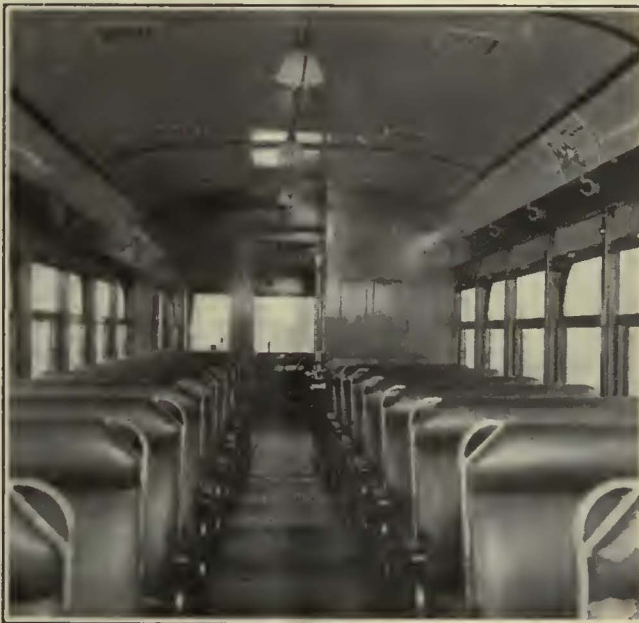
Arched Headlining, Shaded Lamps, Fabrirkold Seats in New Interurban Cars
