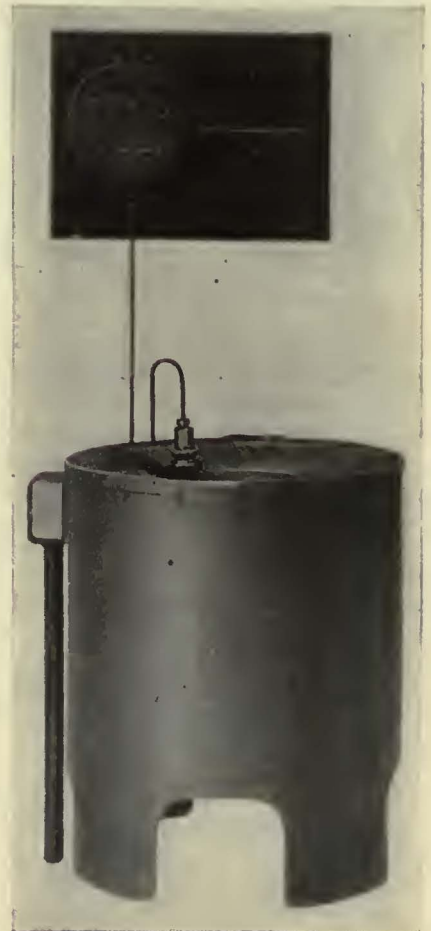
New Automatically Controlled Electric Melting Pot
