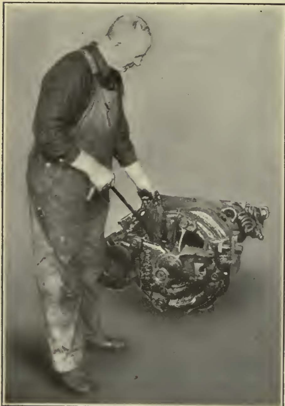
At Left—Packing a Railway Motor Bearing Correctly, Showing How the Wick Should Be Put in Place. At Right—A Correctly Packed Pinion End Housing. The Outer Shell Has Been Cut Away to Show the Wick in Place
