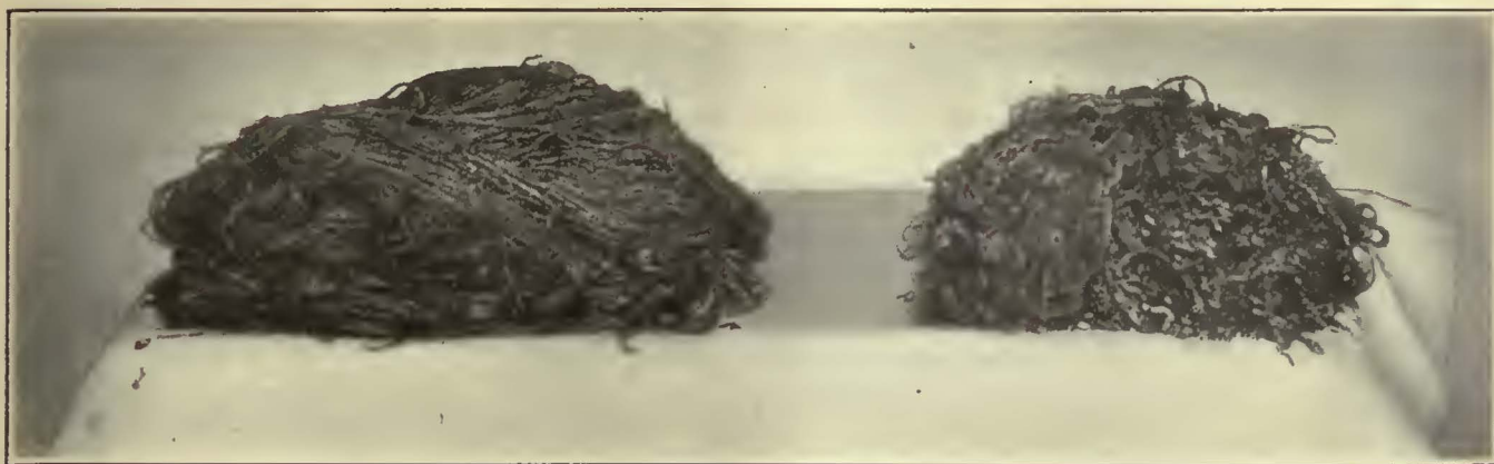
Amounts of Waste Taken from Bearing Housings—at Left, from a Correctly Packed Housing; at Right, from an Incorrectly Packed Housing
