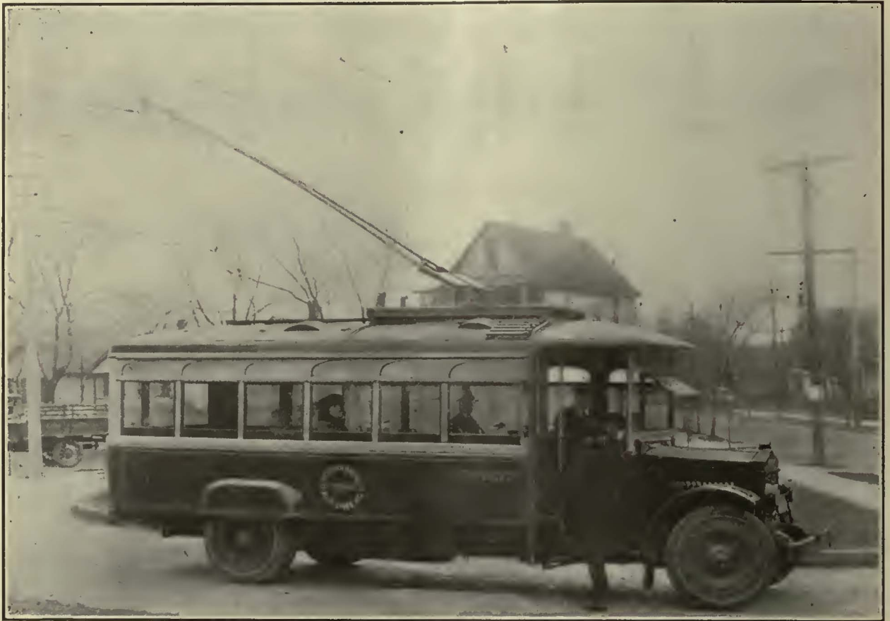
One of nine Brockway Trackless Trolley Cars operated by New York State Railways, Rochester, N. Y.
