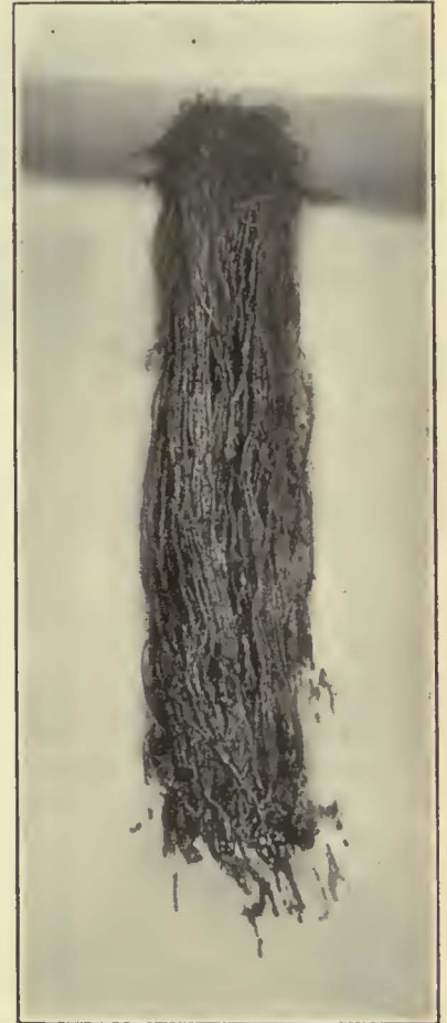
A Long Strand Wool Wick Such as This Should Be Prepared for Feeding Oil to the Bearing Window
