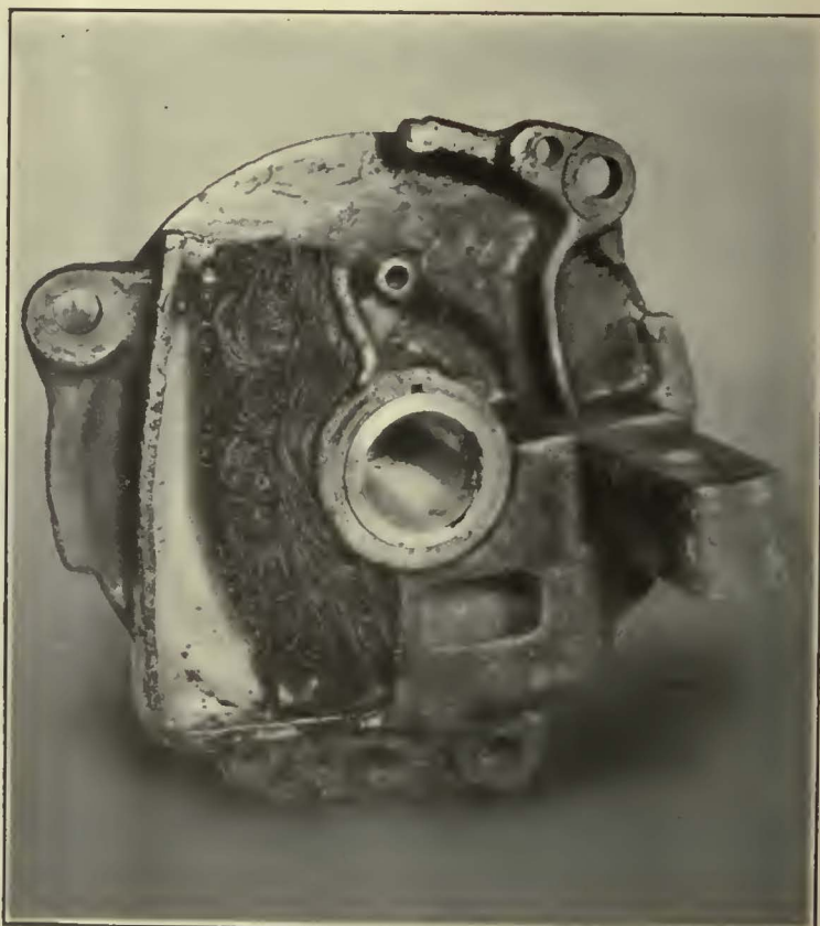
At Left—Packing a Railway Motor Bearing Correctly, Showing How the Wick Should Be Put in Place. At Right—A Correctly Packed Pinion End Housing. The Outer Shell Has Been Cut Away to Show the Wick in Place
