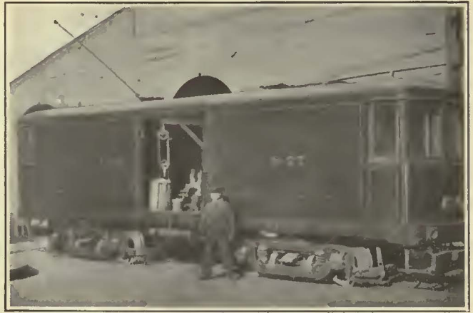
Pony Trucks for Use in Case of Accidents Are Swung Off the Wreck Car by Means of a Derrick
