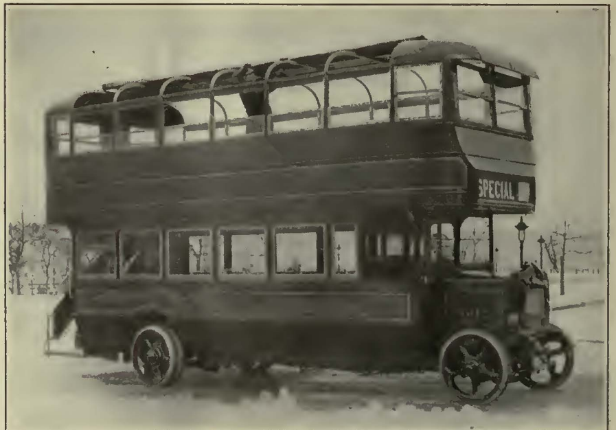
Sixty-four-Passenger Bus with Removable Top Equipped with Roll Roof and Side Curtains. This Arrangement Is Designed to Make the "Open Deck" Usable All Year
