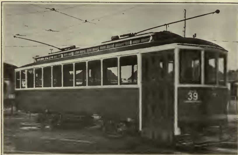
Four Cars of This Type Have Been Converted by the Winnipeg Electric Railway for One-Man Operation on Suburban Lines
