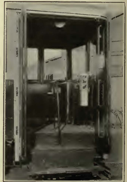
Double Doors, Separately Controlled, and Step Arrangement on Rebuilt Winnipeg Cars
