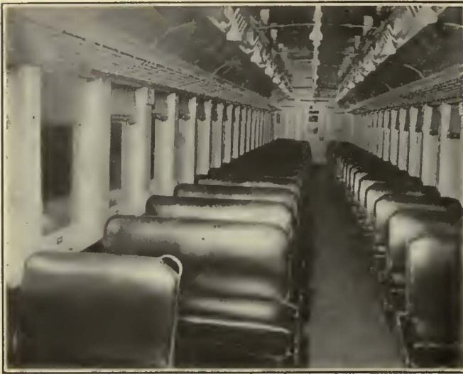
Two Experimental Arrangements of Seats to Increase the Capacity. Left—Back-to-Back Stationary Seats. Right—Reversible Seats
