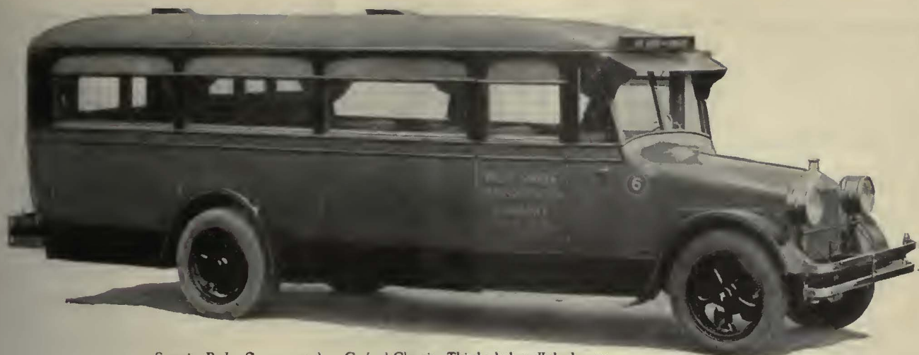
Superior Parlor Car, mounted on Garford Chassis. This body has all the beauty and comfortable seating and riding qualities of the finest De Luxe Coach. Being of the pay-enter type it permits of profitable one man operation without lost time as the operator need never leave his seat at stops to manipulate doors or collect fares.
