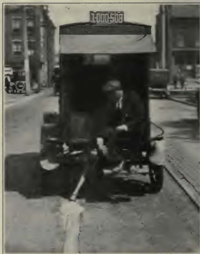
Track in Utica Is Sanded by Means of This Small Auto Truck
