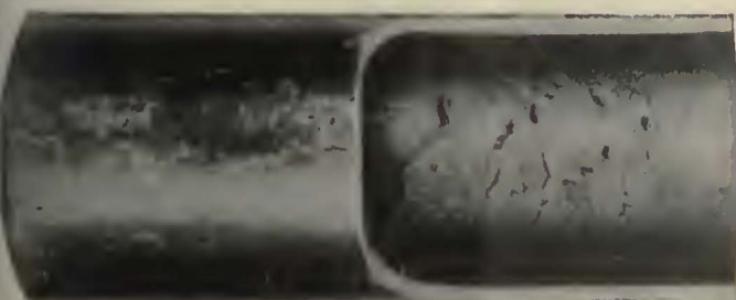
Ordinary black butt-weld pipe showing characteristic coating of welding-scale
