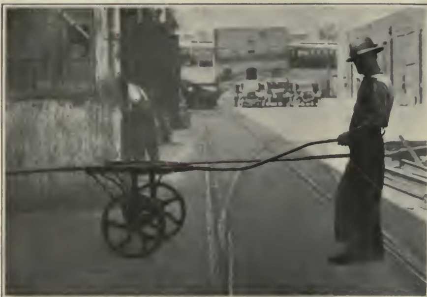
This Two-Wheeled Buggy Has Been Found Useful for Handling Long Bar Material About the Forge Shop of the Kansas City Railways
