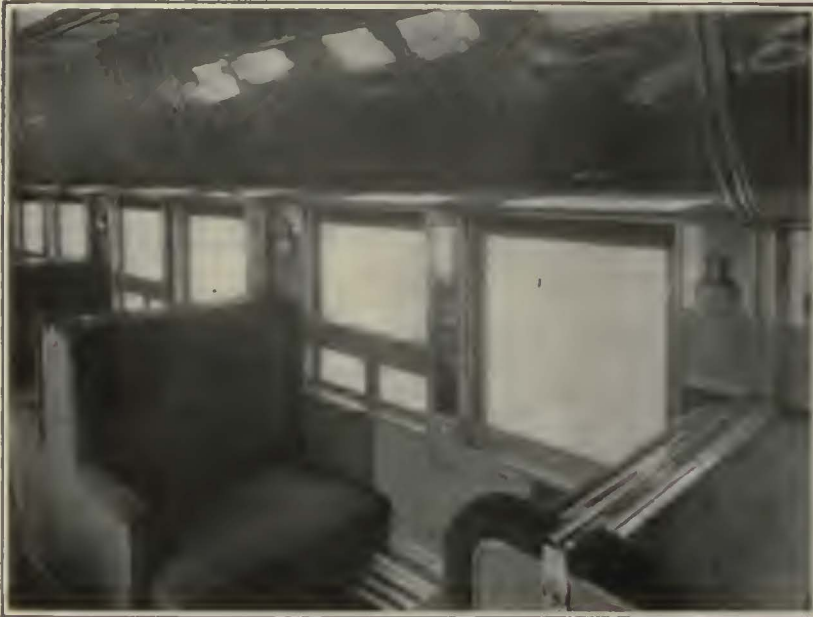
At Left—Each Berth Section Is 6 Ft. 4 In. Long and 3 Ft. Wide and Is Arranged in a Manner Similar to that of a Pullman. At Right—Ventilating Windows for the Upper Berth Are Provided and Two-Section Curtains. In the Foreground Is a Folding Table for Use During the Daytime
