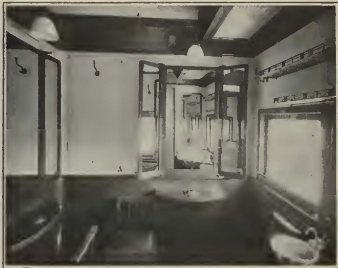
The Ladies' Dressing Room Contains the Latest Appointments, Including Two Sets of Three-Section Swinging Mirrors, Three Chairs, Washbowl and Dental Lavatory
