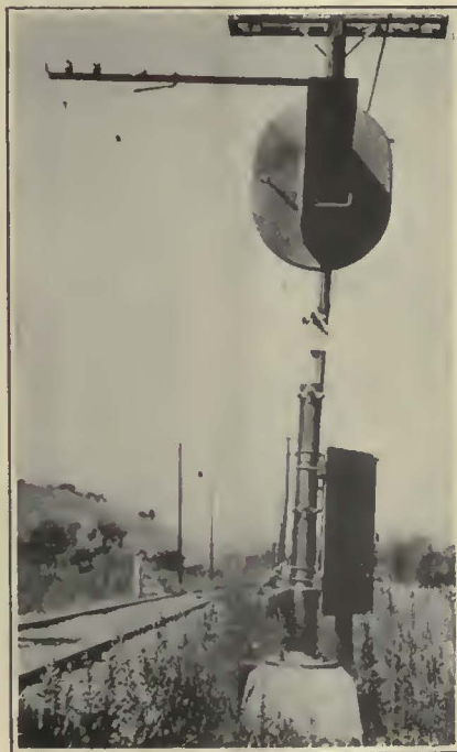
On the San Francisco-Sacramento Railroad Signals of This Type Are Lighted Only in the Block Immediately Ahead of an Approaching Train
