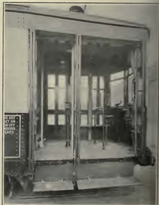
The Automatic Exit Doors Are Controlled by a Treadle in the Platform Floor. Passengers Board Through the Door at the Right and Leave Through the Automatic Exit.
