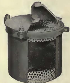
The 8-in. Suction Strainer consists of a cylindrical body with a compact layer of pulled, curled hair between two perforated plates, and is so constructed as to be readily taken apart for cleaning at stated periods.
