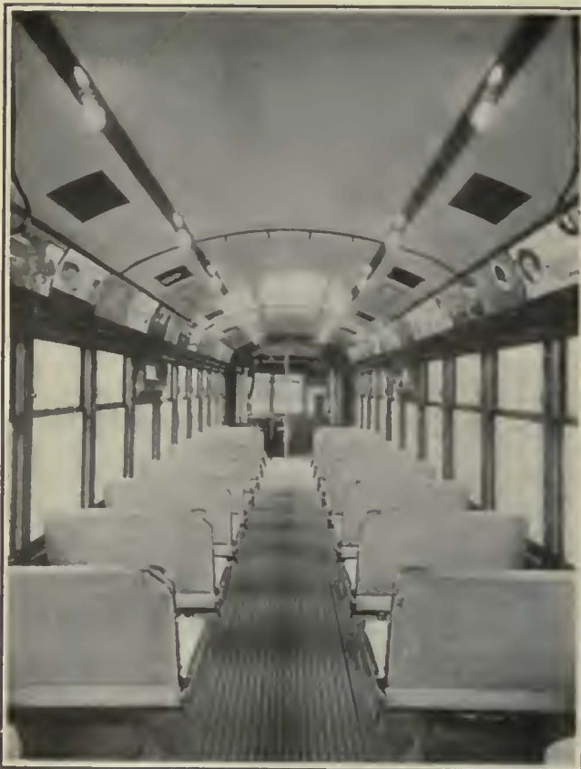
Simple Lines and Smooth Curves with the Dull Finished Cherry Trimming Feature the Interior of This Car. The Wide Aisle Facilitates Passenger Movement.
