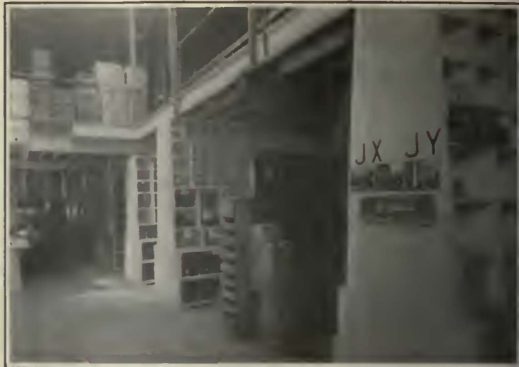
Main Storeroom Showing "Daylight" Cases for Material. The Unit System of Piling Is Used to a Limited Extent. Cases Are Painted White
