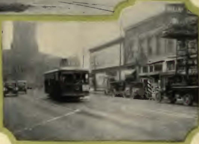
This single-truck Birney safety car, equipped with Safety Car Devices, is the type that helped build patronage for the Northern Texas Traction Company.
