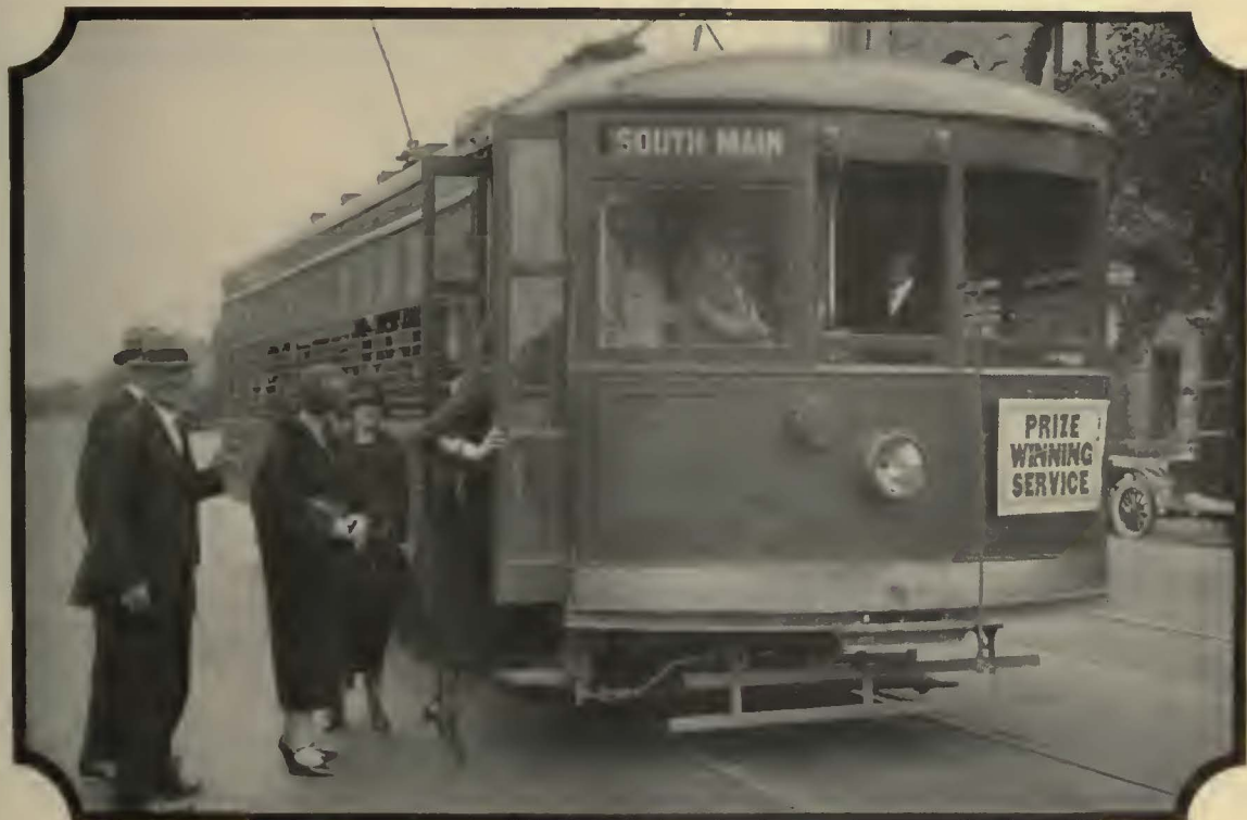
One of the Northern Texas Traction Company's new Birney Safety Cars on which H-B Life Guards are standard equipment.
