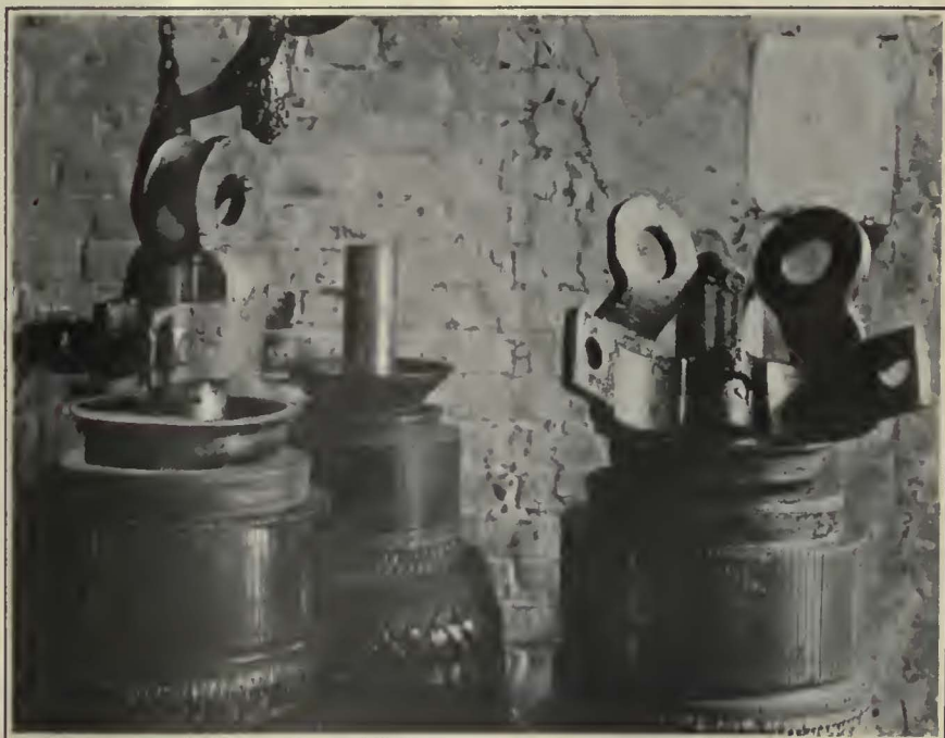
This Clamp Is Used at Kansas City to Handle Armatures in a Vertical Position for Dipping and Baking
