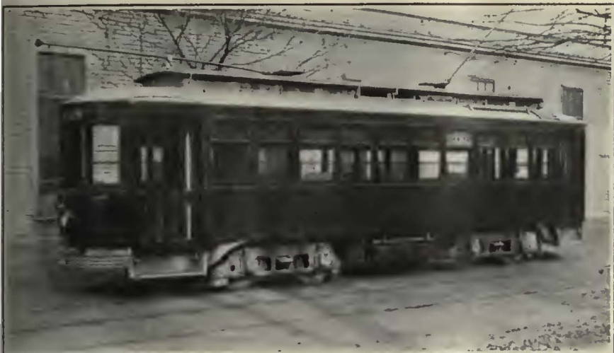
The Cost of Car Painting Has Been Reduced by the Use of a Simplified Color Scheme Without Striping or Lettering
