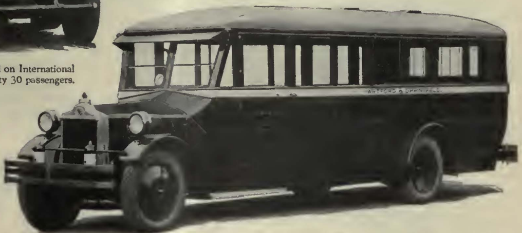
Superior De Luxe Pay-Enter body mounted on a Guilder chassis. Seating capacity 25 passengers.
