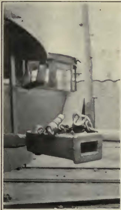
At Left, Old Coupling Head Which Protruded Beyond the End of the Car. At Right, the New Coupling Bar Does Not Extend Beyond the Bumper
