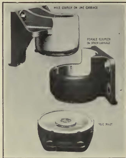
Details of Articulation Connections, London & North-Eastern Car
