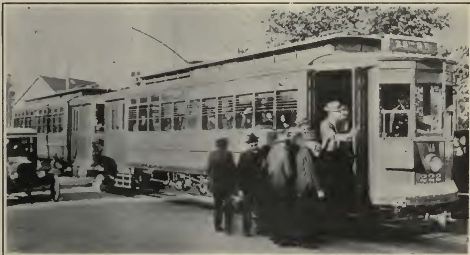
Recent Type of Milwaukee Articulated Car, Using Drum Connection
