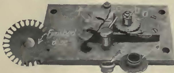
Fig. 2. Equally Spaced Slots in Fish Paper Insulating Disks for Fan Motor Armatures Are Cut in This Indexing Die
