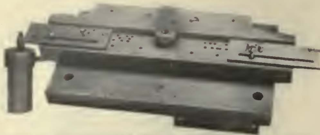
Fig. 12. The Holes in Various Types of Controller Cylinder Segments Are Located in This Adjustable Jig
