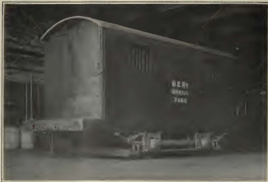
This Car Carries a Complete Outfit of Painters' Supplies and Provides a Place Where the Men Can Change Their Clothes
