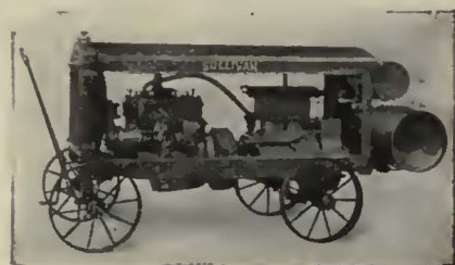
163-ft. "WK-311" Compressor, on Steel Wheel Truck.
