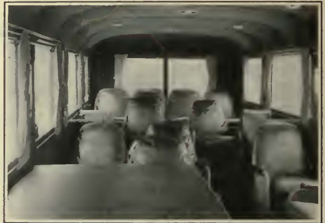
A Folding Table Makes It Possible to Utilize This Bus as an Office While en Route
