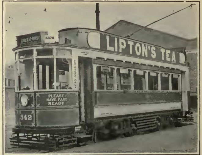
This New Single-Deck One-Man Car Is Being Tried Out on the London United Tramways
