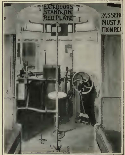
At Left, the Car Interior Resembles Those in Use on American Street Railways. At Right, Automatic Devices Used Include an Unlocking Exit Door, a Dead Man's Handle for the Brakes and a Ticket-Issuing Machine
