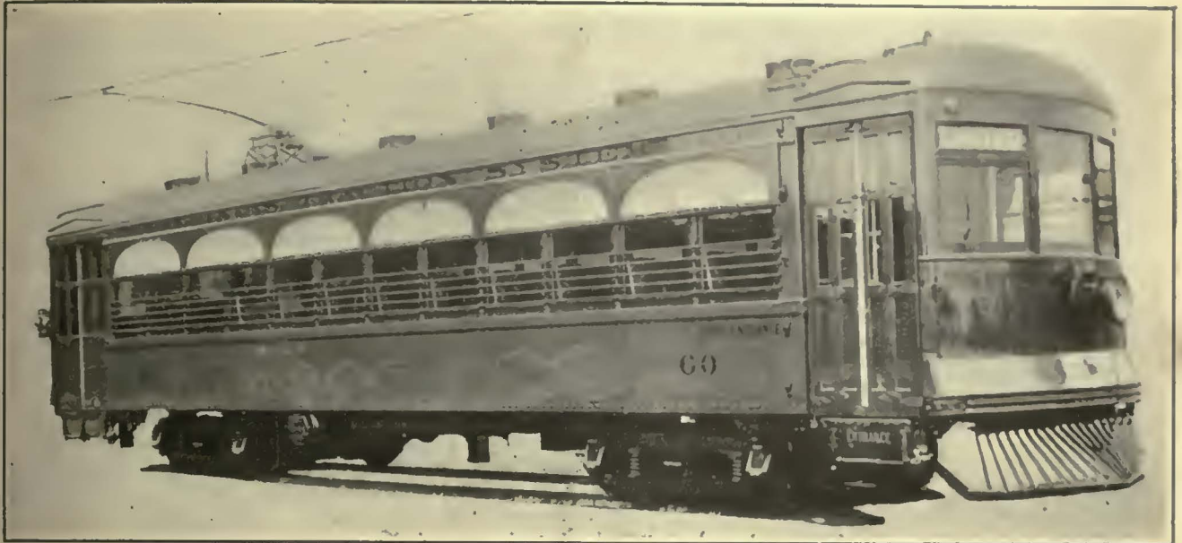
Double-Arched Windows Give the Exterior an Attractive Appearance. The Rear Folding Doors Are Used for Loading Baggage, but a Step Is Provided so that Passengers at Busy Terminals May Board or Alight at Both Ends
