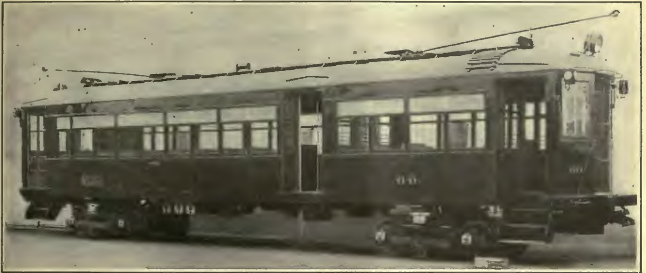
This Philadelphia & Western Car Is Divided Into Two Compartments. Center Doors Without Steps Are Provided
