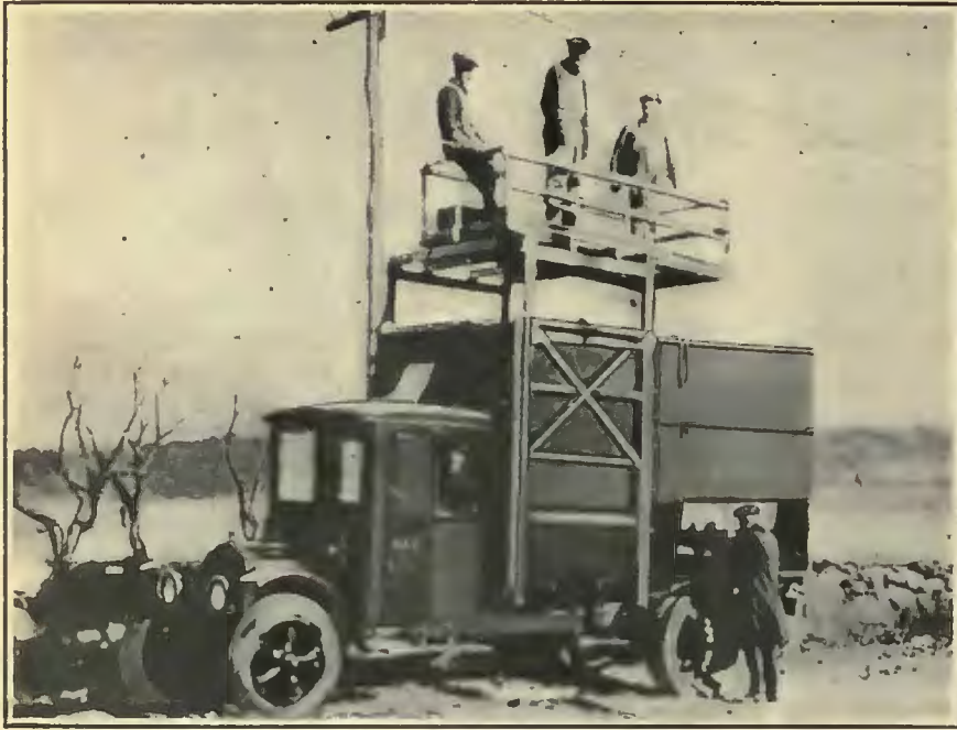
A Permanently Inclosed Body Is a Feature of This Heavy Tower Truck
