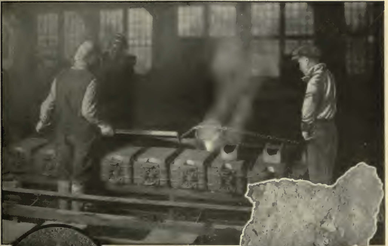
Foundry slag skimmed from molten bronze
