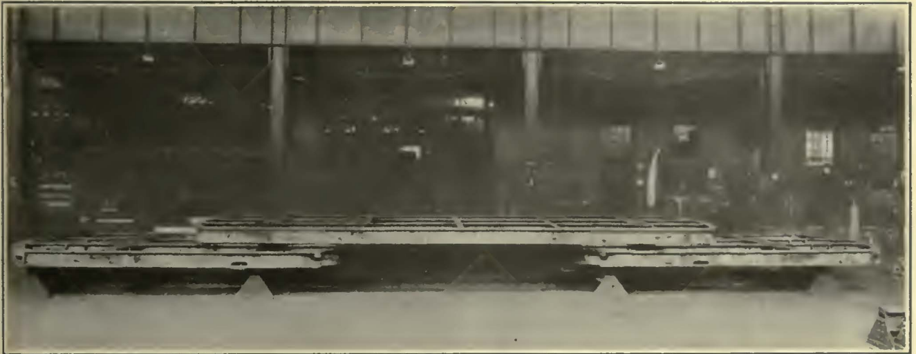
The Three Cast-Steel Frames for One Complete Unit Are Shown Here in Their Relative Positions
