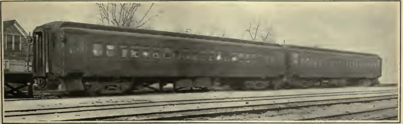
New Illinois Central Cars Similar to These Will Operate on the 1,500-Volt D.C. Circuit in Chicago Suburban Service. A Motor Car and a Trail Car Are Semi-Permanently Connected to Form a Unit. A Train Is Made Up of from One to Five Units
