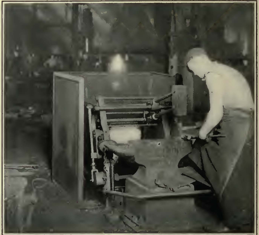
Mechanical Helper In Use at the Morris Park Shops of the Long Island Railroad
