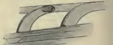
Above is shown the old style cross grain section formerly used. Lack of strength and clumsiness is evident. Note the irons for bracing. These are not needed with the new construction. This is one place where weight is saved.
