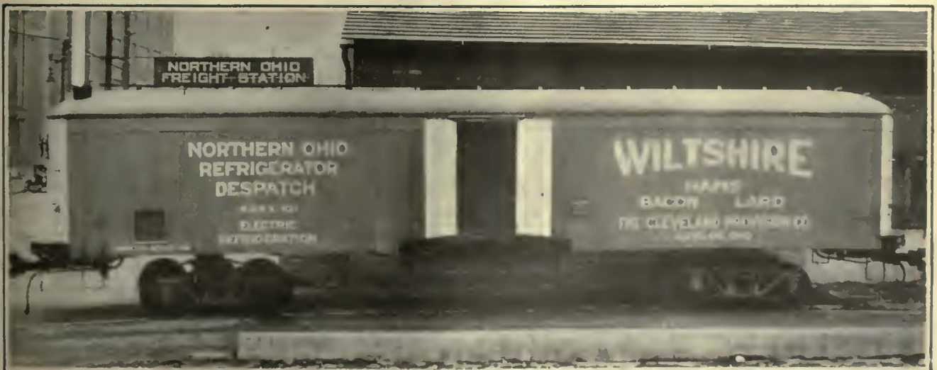
An Electrically Cooled Refrigerator Car that Has Been Placed in Service on the Northern Ohio Traction & Light Company's Interurban Lines
