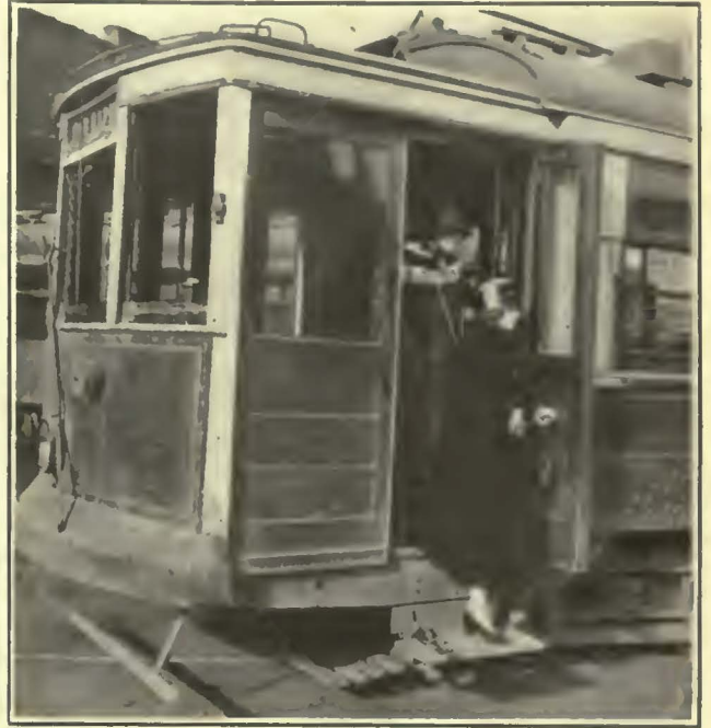
When the Last Alighting Passenger Clears the Step the Rear Exit Door Automatically Closes
