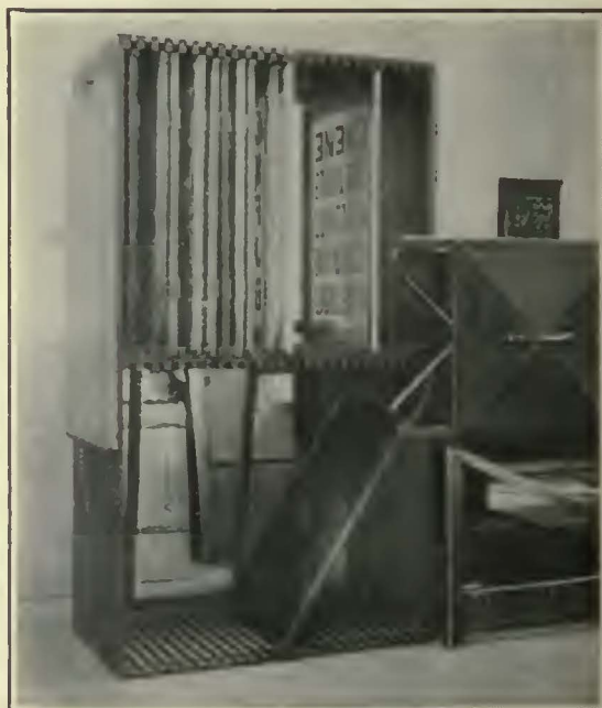
Signs Are Printed on the Handy Table Shown at the Left, and When Not in Use Stencils Are Stored in Convenient Racks Shown at the Right
