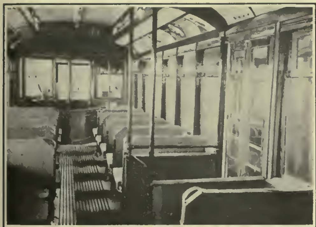
Front-Entrance and Center-Exit Arrangement on the Rebuilt Denver One-Man Cars. Note the Low Partition Which Incloses the Operator's Position
