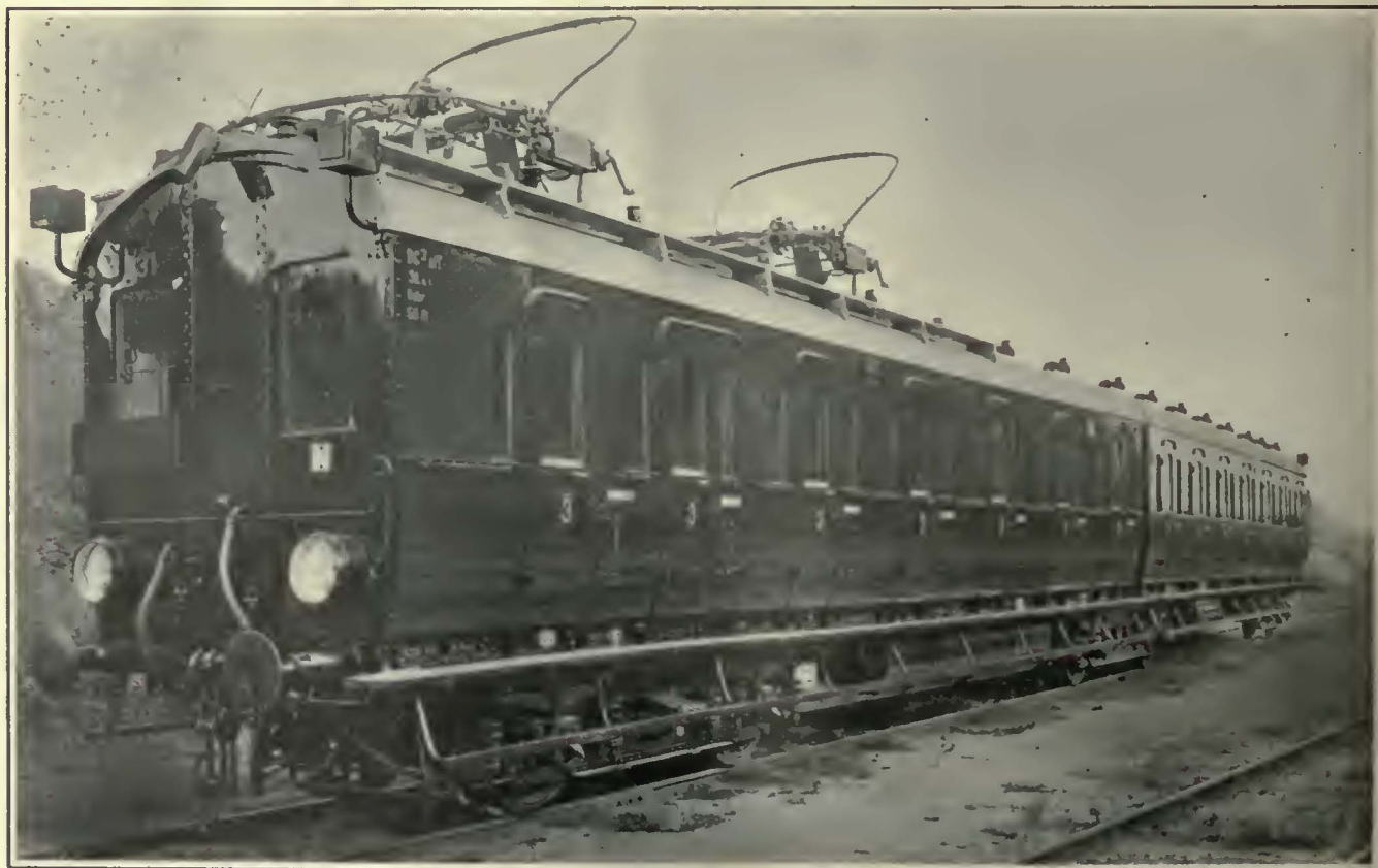
This Two-Car Articulated Train Is Used in Hamburg Suburban Service on the Single-Phase System
