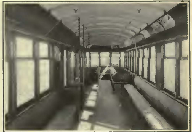
An Interior View of the Dayton Car After Rebuilding Cross-seats were put into the rear section to induce passengers to move back from the front entrance. All piping and control wiring are installed under the longitudinal seats.
