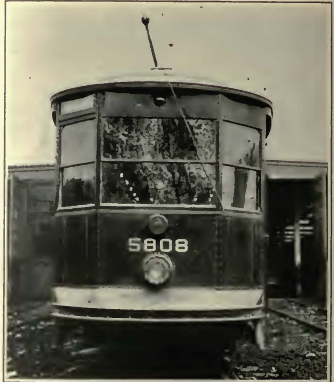
Narrow Window Posts and Metal Sash Have Increased the Vestibule Window Area on This Car
