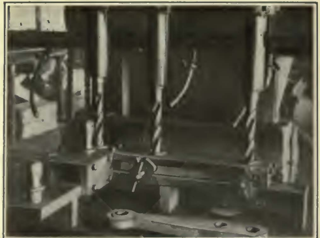
At Left, Simple Jig Holds Air Brake Cylinder Lever While Three Holes Are Drilled Simultaneously. At Right, Where the Holes Are Closer than the Minimum Spacing of Spindle Centers an Angle Jig Allows the Full Machine Capacity to Be Used by Drilling Two Holes in One Lever While the Third Is Being Drilled in Another
