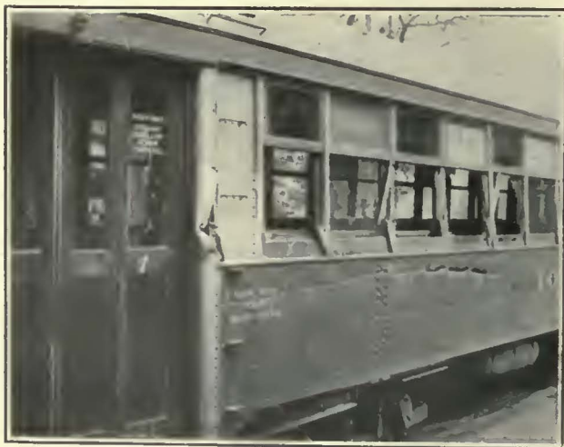
An Oxyacetylene Torch, in the Hands of a Skilled Operator, Made Possible a Substantial Saving in Cost of Repairing This Damage. At left, the car as it came in after an accident. At right, use of the welder eliminated the necessity of removing the damaged side plate
