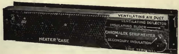
Truss Plank Heater Showing strip element in place and Air Duct.
