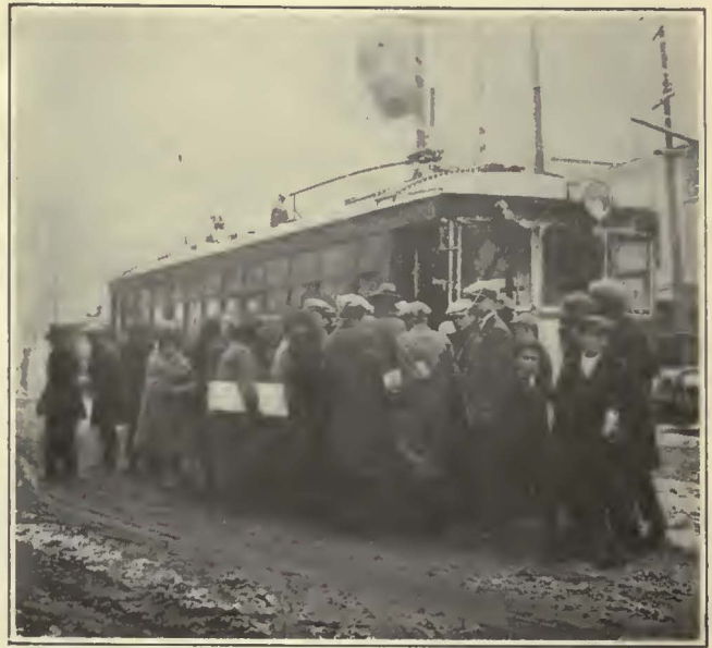
Although One-Man Operation Is Used, These 58 Passengers Were Loaded and Fares Collected from Those Without Tickets in One Minute 23 Seconds
