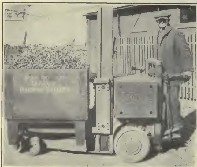
Picking Up a Box of Machine Shop Turnings Preparatory to Delivering It to the Scrap Storage
