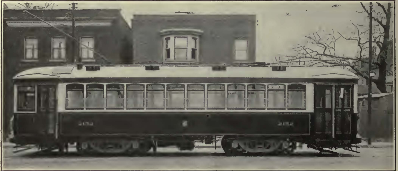
Front-Entrance, Automatic Rear-Exit Car as Remodeled by Toronto Transportation Commission from Rear-Entrance, Pay-as-You-Enter Car
