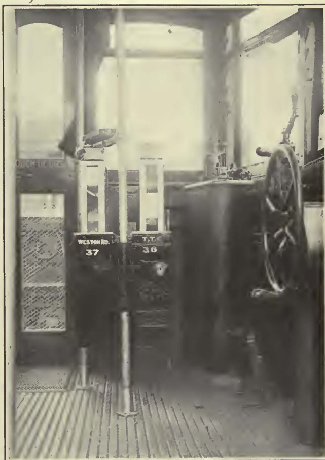
Twin Fare Boxes Are Used to Permit Separate Accounting on One-Man Cars on Weston Road
