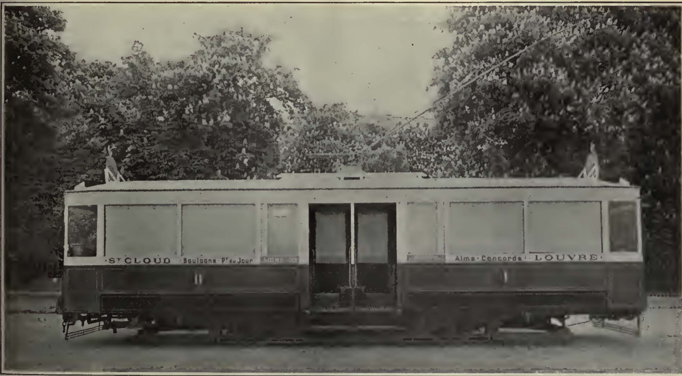
Light-Weight Car of the T.C.R.P., with Motors Mounted on the Body Framing and Axles Attached to the Body by Springs and Shackles. This Arrangement Gives About 15-In. Play for the Axles
