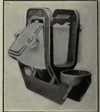
The Saddle Swings from the Top of the Journal Box to Permit Lateral Movement of the Axle
