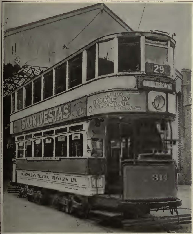
Double-Deck Double-Track Car of the Metropolitan Electric Tramways Is Typical of Many English Cars
