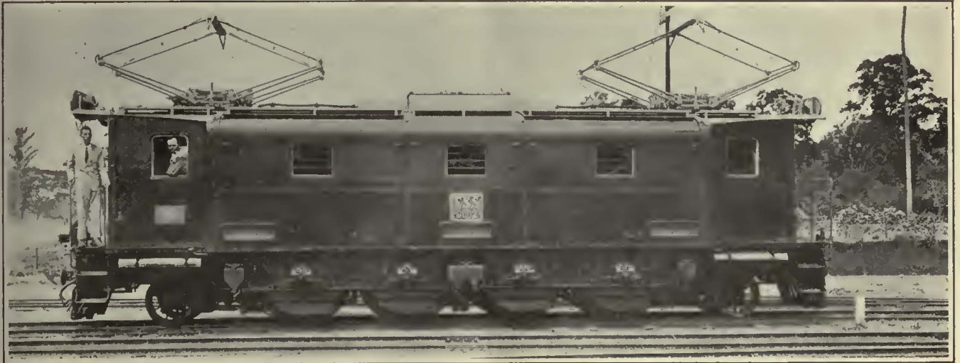
This is a 1,500-Volt Express Train Locomotive Built in Switzerland for the Java Electrified States' Railways
