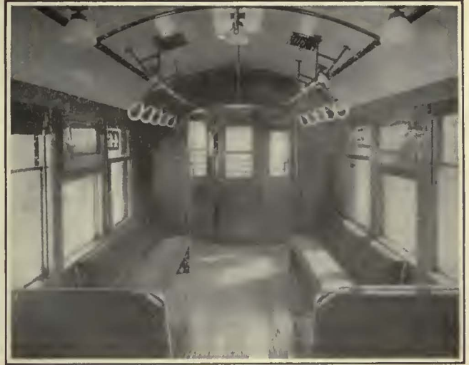
Short Longitudinal Seats at the Doorways Help to Prevent Congestion by Providing a Wide Aisle at Ends
