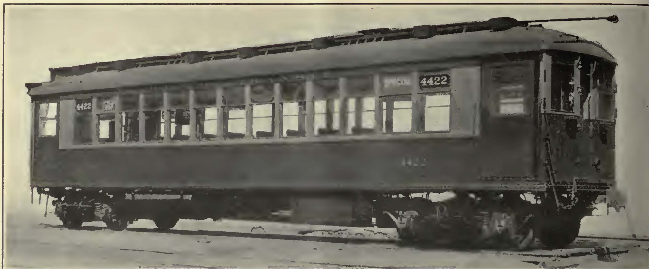
One of the New Cars. Steps Are Unnecessary Because High Level Platforms Are Used at All Stations
