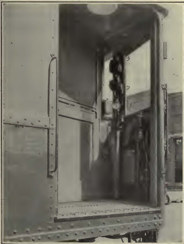
At Left—Motorman's Compartment Is Located at the Front Right-Hand Side of the Car. When Not in Use It Is Made a Part of the Vestibule by Closing the Door to Conceal the Operating Equipment. At Right—The Switch Panel Is a Completely Inclosed Unit on the Platform
