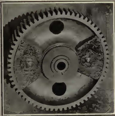
Pads of Rubber-Asphalt Material Bolted to Web of Gear Have Been Found Effective for Reducing Gear Noise
