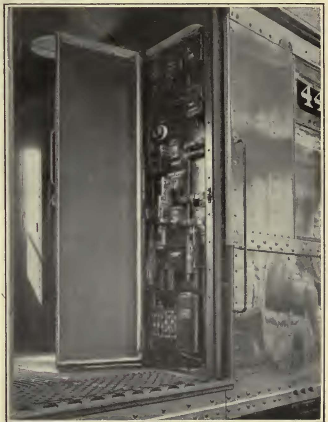
At Left—Motorman's Compartment Is Located at the Front Right-Hand Side of the Car. When Not in Use It Is Made a Part of the Vestibule by Closing the Door to Conceal the Operating Equipment. At Right—The Switch Panel Is a Completely Inclosed Unit on the Platform
