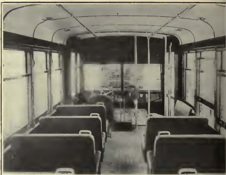
At Left, Driving Mechanism Consists of Westinghouse Type V-91 Motors Mounted on a Figeol Chassis. At Right, Interior of the Body, Built by the American Car Company, Closely Resembles that of the Typical Birney Car
