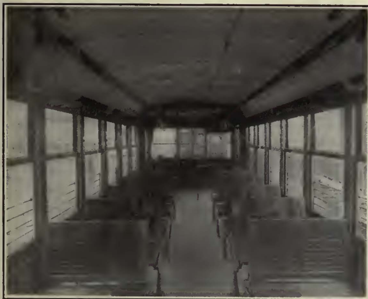
At Left—The Interior Finish Is of Mahogany. Ten Reversible Seats Are of Wood Slat Construction. At Right—A Book Type Folding Seat Provides Additional Seating on the Rear Platform
