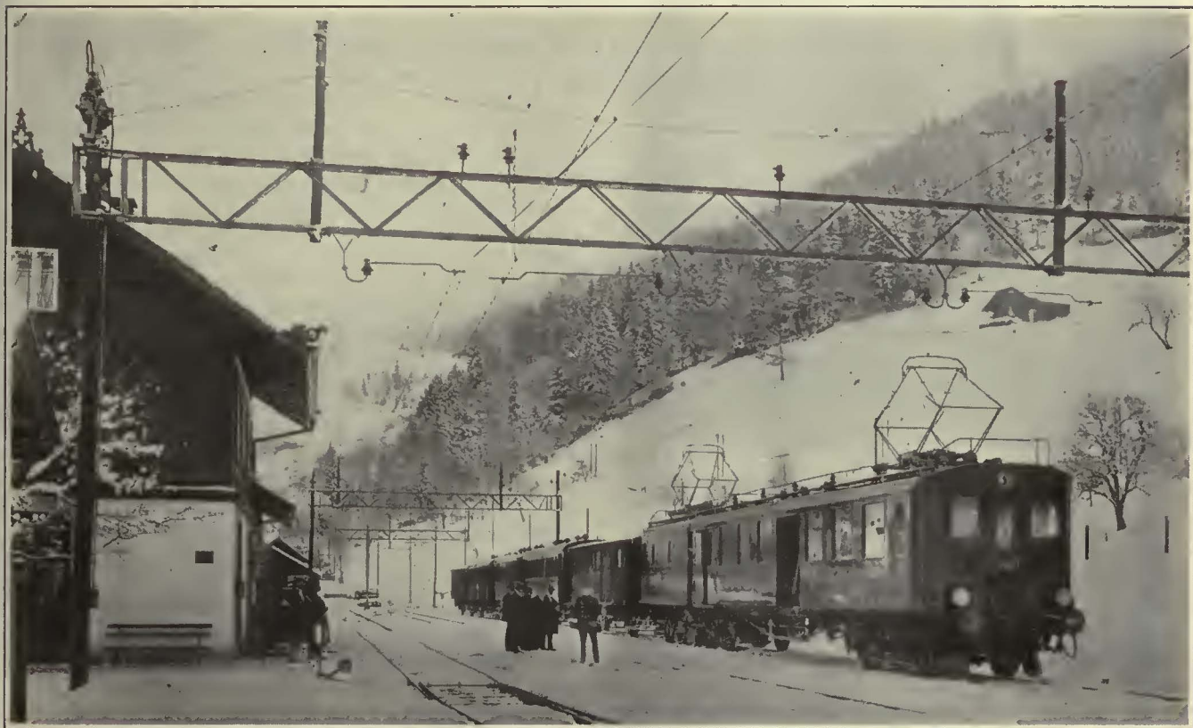
Combination Twelve-Wheel Locomotive-Car Used in Switzerland on Runs Where Traffic Does Not Justify Regular Train Operation
