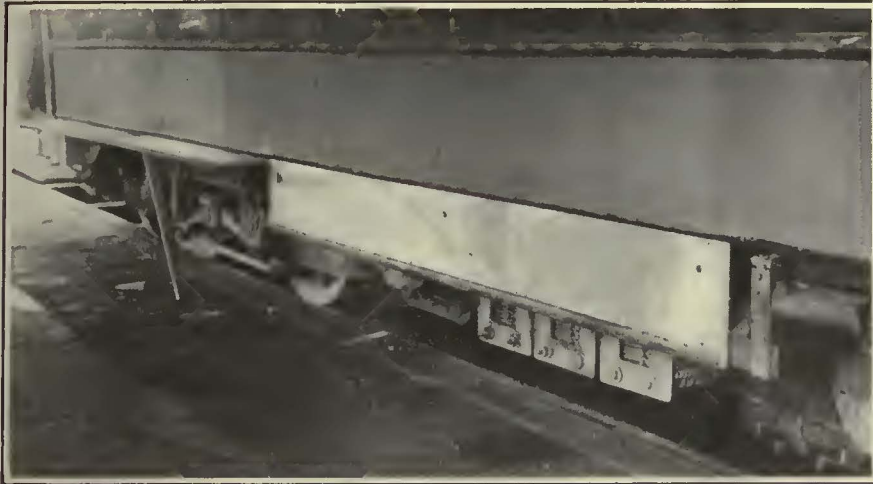
Metal Moldings at Top and Bottom of Hinged Aprons Give Finished Appearance and Add Streamline Effect
