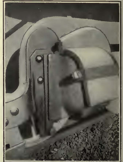
Shims Bolted to the Truck Frame Save Wear on the Journal Box on Cars of the Union Street Railway
