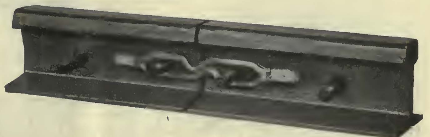
Type E Brazed Bond for bonding around the joint, or around special work. This bond is also applicable to installation on the top of the rail base.
