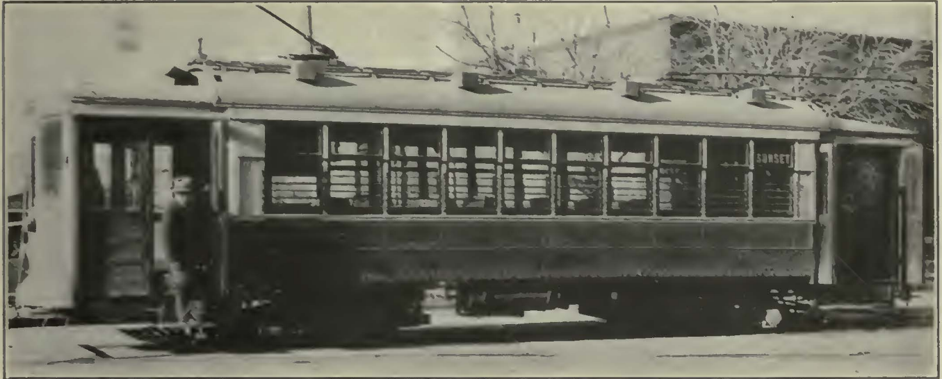
Exterior of Earlier Type of Car, 50 of Which Will Be Changed Over for One-Man Operation. Complete One-Man Safety Features Will Be Used and Automatic Treadle Equipment Will Allow Rear Exit Operation
