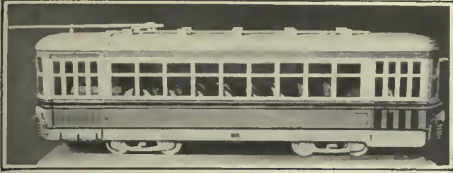
Fig. 4—Side View with Latest Changes By carrying the same colors in the same width bands across the doors, a longer effect to the car body is produced.
