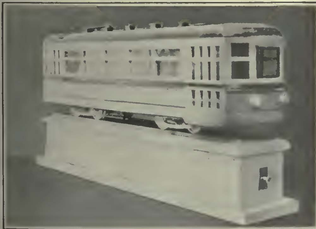
Fig. 7—Door Side of Model Car with Large Windows While large windows may be an added convenience for passengers inside the car, they detracted from long flowing lines which are now being sought in car construction.
