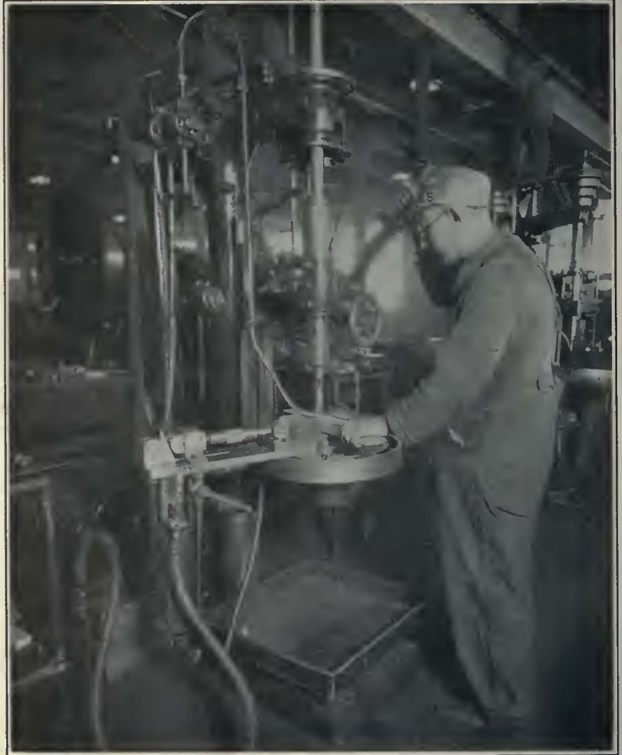
Air-Operated Chuck and Liquid Circulating System as Applied to a Drill Press in the Shops of the Department of Street Railways, Detroit
